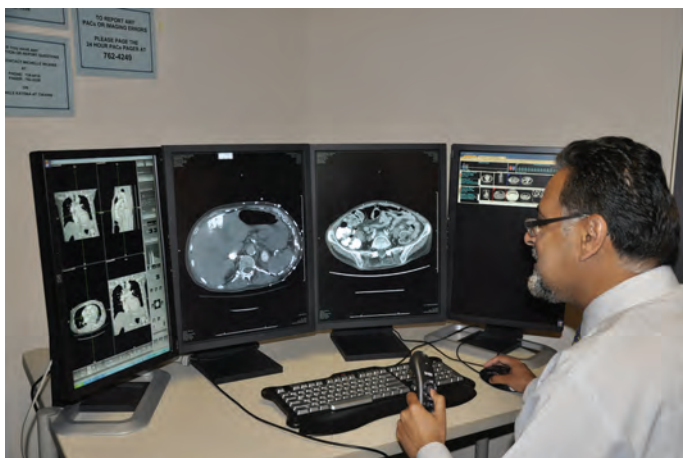
■ FIGURE 5-26 Interpretation workstation containing two 1.5 by 2 k pixel (3 megapixel) portrait-format grayscale monitors for high resolution and high luminance image interpretation, flanked by two 1.9 by 1 k (2 megapixel MP) color “navigation” monitors ( left and right ) for PACS access, patient worklist, timeline, and thumbnail image displays; multipurpose display for 3D color rendering, digital voice dictation reporting, and EMR and RIS information access. The keyboard, mouse, and image navigation and voice dictation device assist Ramit Lamba, M.D., in his interpretation duties.
