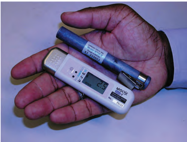
■ FIGURE 21-8 Examples of analog and digital pocket dosimeters. Pocket ion chamber courtesy of Arrow-Tech, Inc. Rolla, ND, and electronic personnel dosimeter courtesy of Cone Instruments, Solon, OH.
