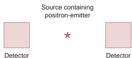
■ FIGURE 19-24 Point source of a positron-emitting radionuclide, in air, midway between two identical detectors.
