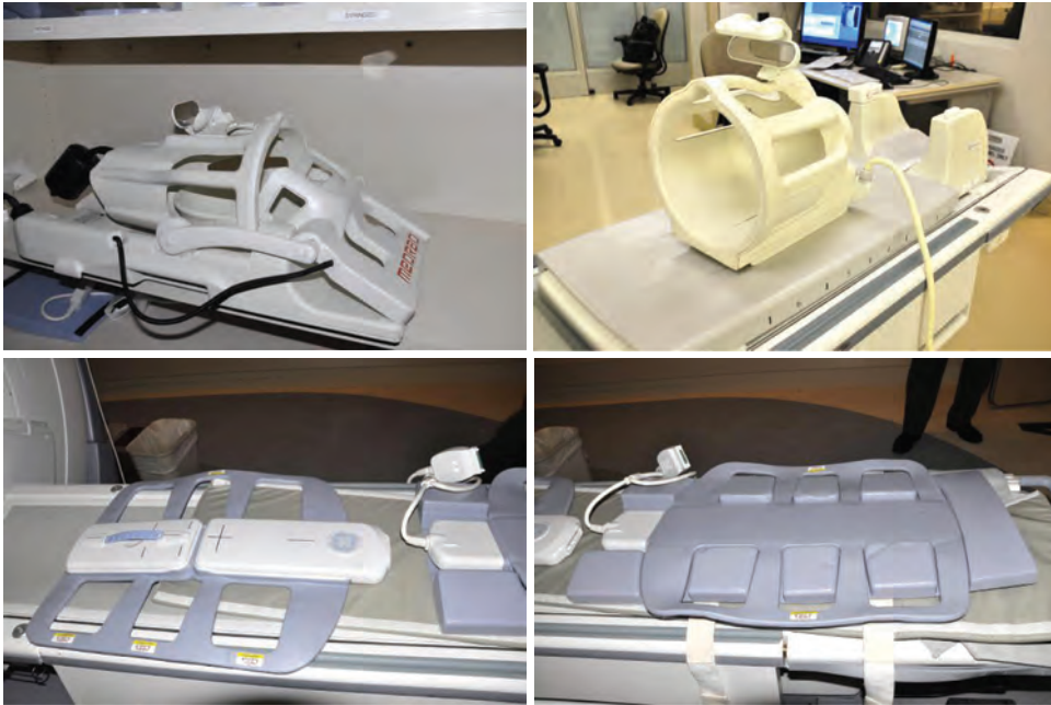
■ FIGURE 13-41 Radiofrequency surface coils improve image quality and SNR for specific examinations. Upper left is a dedicated head and neck coil. Upper right is a dedicated head coil; the lower left and lower right images illustrate the two components of an 8 channel phased array coil for body imaging.
