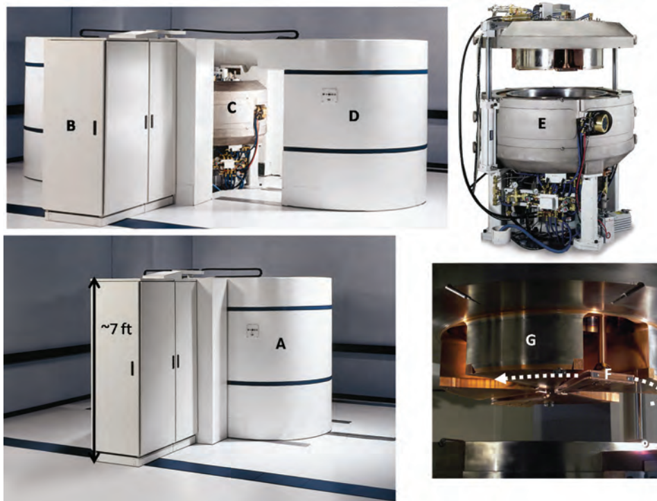
■ FIGURE 16-3 Commercial self-shielded cyclotron for radionuclide production capable of producing a 60 \mu A beam of protons accelerated to \sim 11 MeV is shown with the radiation shields closed (A). Designed with a small footprint to fit into a relatively small room ( 24' \times 23' \times 14' height) (B) Power supply and control cabinet (C) Cyclotron assembly approximately 10,000 kg (22,000 lb) (D) Retractable radiation shielding (open) approximately 14,500 kg (32,000 lb) of borated concrete and polyethylene. Neutrons and gamma radiation are an unavoidable byproduct of the nuclear reactions which are used to produce the desired radioactive isotopes. Boron and polyethylene are added to the radiation shield to absorb neutrons. The shielding is designed so that radiation exposure rates are reduced to the point where technologists and other radiation workers can occupy the room while the accelerator is in operation (less than 20 \mu Sv/h at 24 ft from the center of the cyclotron). (E) Cyclotron assembly open. Hydrogen gas line at the top of the cyclotron assembly provides the source of hydrogen ions to be accelerated. (F) One of four cyclotron dees. The acceleration potential is supplied by high frequency voltage. In this system, four dees provide eight accelerations per orbit, thus reducing acceleration path length and beam loss. (G) Beam shaping magnets act as powerful lenses to confine ions to the midplane. The dotted white arrow shows the beam path through one of the dees.
