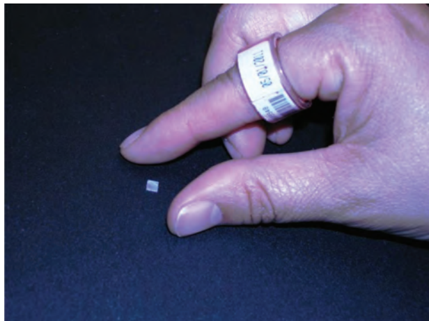
■ FIGURE 21-5 A small chip of LiF ( right ) is sealed in a finger ring (underneath the identification label). In nuclear medicine, the ring is worn with the LiF chip on the palmar surface such that the chip would be facing a radiation source held in the hand.
