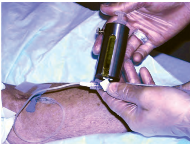
■ FIGURE 21-18 A butterfly needle and three-way stopcock connected to a syringe with normal saline and a syringe shield containing the syringe with the radiopharmaceutical for injection. The barrel of the syringe shield is made of a high- Z material (e.g., lead or tungsten) in which a leaded glass window is inserted so that the syringe scale and the contents of the syringe can be seen.
