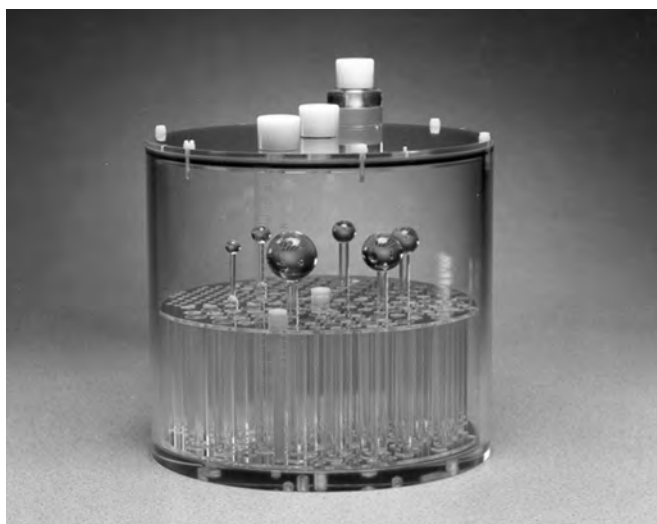
■ FIGURE 19-13 "Jaszczak" phantom for testing SPECT systems, a product of Data Spectrum Corporation. (Photograph courtesy Data Spectrum Corporation.) A soluble radioactive material, typically labeled with Tc-99m, is introduced into the phantom and mixed in the water until it is uniformly distributed. The acrylic plastic spheres and rods are not radioactive and are "cold" objects in the radioactive solution.
