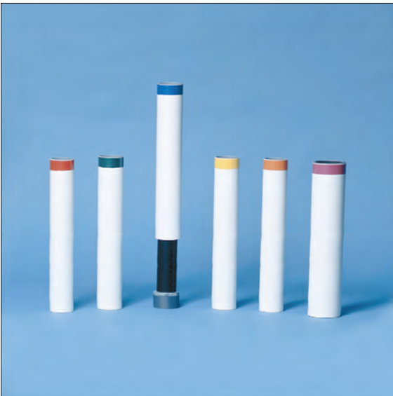
■ FIGURE 17-27 Set of cylindrical lead sleeves used to test dose calibrator linearity. These color-coded sleeves of different thicknesses use attenuation to simulate radioactive decay over periods of 6, 12, 20, 30, 40, and 50 h for ^{99\text{m}}\text{Tc} . Additional sleeves are available that can extend the simulated decay interval up to 350 h. Photo courtesy of Fluke Biomedical Radiation Management Services, Cleveland, Ohio.
