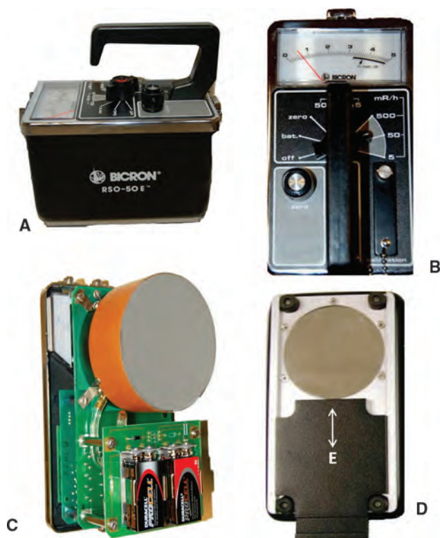
■ FIGURE 17-6 Portable air-filled ionization chamber survey meter (A). This particular instrument measures exposure rates ranging from about 0.1 mR/h to 50 R/h. The exposure rate is indicated by the position of the red needle on the scale. The scale is selected using the range knob located below the scale (B). In this case, the needle is pointing to a value of 0.6 on the scale, and the range selector is set at 50 mR/h. Thus, the exposure rate being shown is 6 mR/h. The interior of the instrument is shown (C) and the ion chamber, covered with a thin Mylar membrane, is easily seen. On the bottom of the meter case (D) is a slide (E) that can cover or expose the thin Mylar window of the ion chamber. This slide should be opened when measuring low-energy x-ray and gamma-ray radiation. The slide can also be used to determine if there is a significant beta radiation component in the radiation being measured. If there is no substantial change in the measured exposure rate with the slide open (where beta radiation can penetrate the thin membrane and enter the ion chamber) or closed (where the ion chamber is shielded from beta radiation), the radiation can be considered to be comprised primarily of x-rays or gamma rays.
