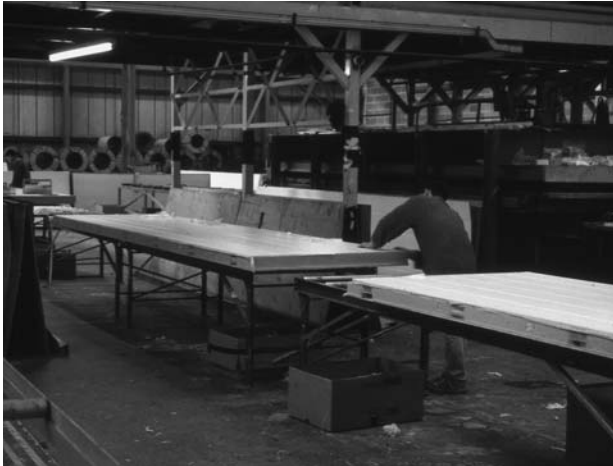
6.16 Batch production of foamed panels – horizontal foaming.
