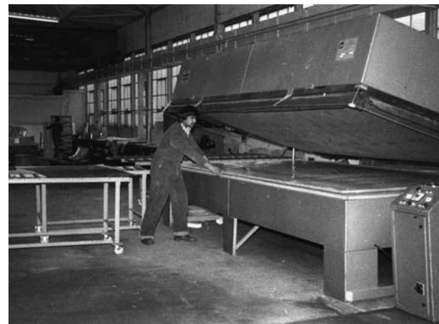
6.19 Laminated panel production using vacuum presses.
