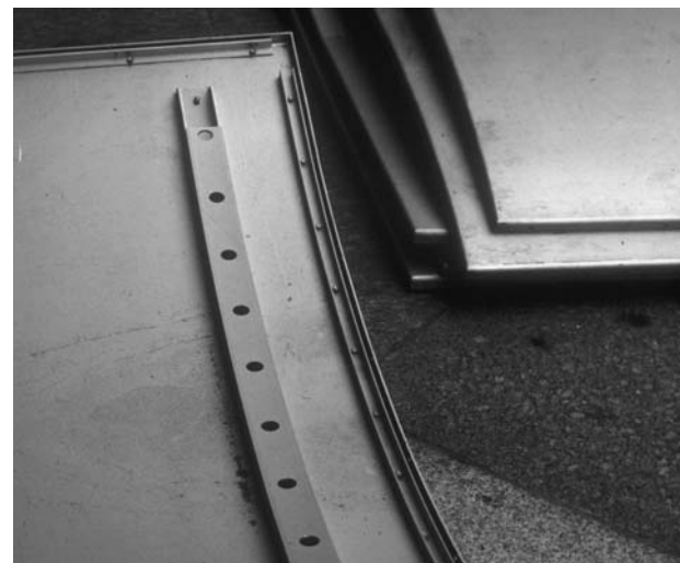
6.24 Stiffening angles to rolled sheet panel.
