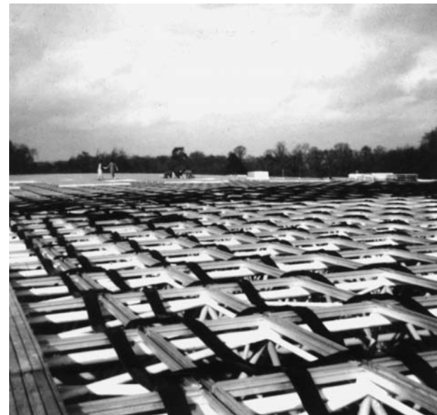
6.9 Lattice gaskets used at Sainsbury Centre.
