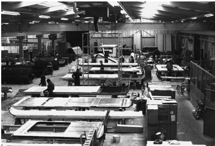
3.6 Typical GRP production with large curing box at the rear of the factory.
