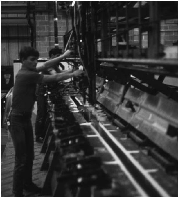
6.17 Batch production of foamed panels – vertical foaming.
