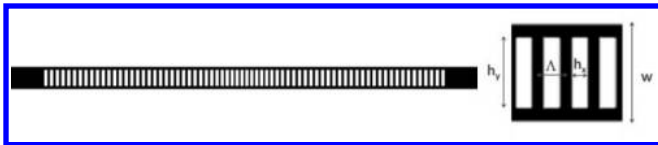
Figure 6.5 Geometry of the 1D optomechanical structure as seen from the top. On the right we show a zoomed region illustrating the different geometric parameters characteristic of this particular design.
