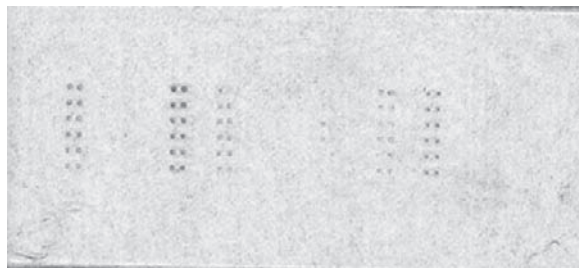
FIG. 3.3. DNA chip after labeling with gold nanoparticles and subsequent silver enhancement. The spots show gold nanoparticles specifically bound by DNA–DNA hybridization and clearly visible through their dark color after silver deposition onto the particles.
