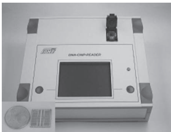
FIG. 3.9. DNA chip reader for fast and automated readout of DNA chips ( inset ) with electrical detection.
