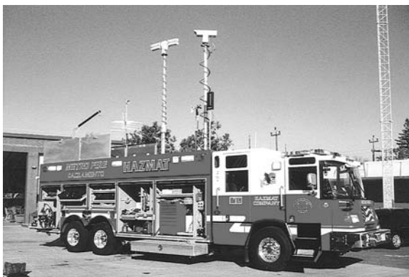
Figure 10.7 (See color insert following page 236.) Sacramento County Fire Department’s new hazmat unit with closed circuit television, complete analytical laboratory, light towers and other typical hazmat equipment.
