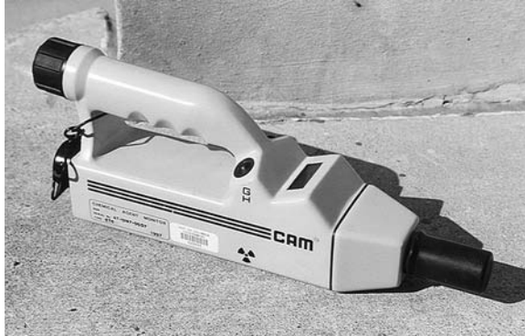
Figure 8.6 Chemical Agent Monitor (CAM).
