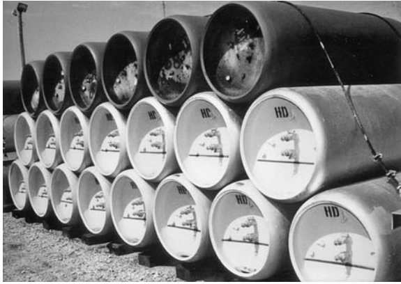
Figure 1.5 One-ton containers of HD mustard agent stored at one of the chemical stockpile sites in the U.S. awaiting destruction. (Source: U.S. Army.)
