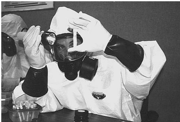
Figure 8.12 During training at the Center for Domestic Preparedness (CDP) in Anniston, AL, an emergency responder in Level C protective clothing uses a flashlight to better view turbidity in a test sample.
