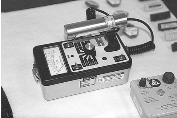
Figure 6.6 All response organizations should have a radiological monitoring instrument in order to scan for radioactive materials at an incident scene.
