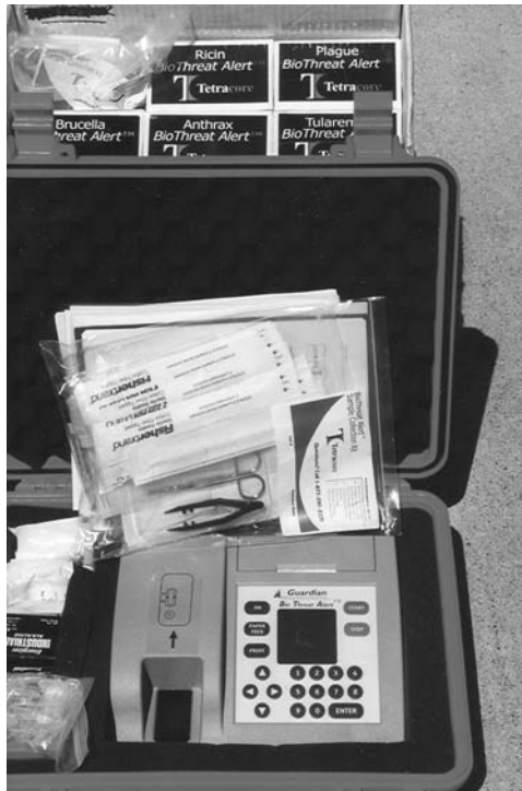
Figure 8.13 Tetracore Guardian biological test kits with reader for ricin, plague, tulaemia, anthrax, and brucella.
