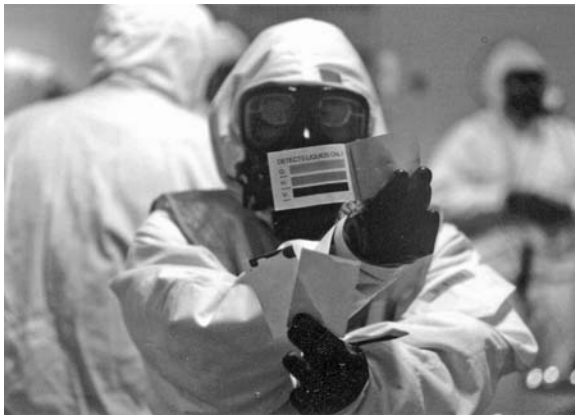
Figure 8.10 Responder in proper protective clothing using M-8 paper and comparing results to chart inside front cover.
