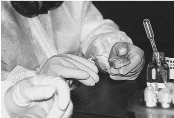
Figure 8.9 A CDP student using a test strip to check for protein content compares his findings to a container comparison chart. Determining protein content helps emergency responders evaluate suspect powders.
