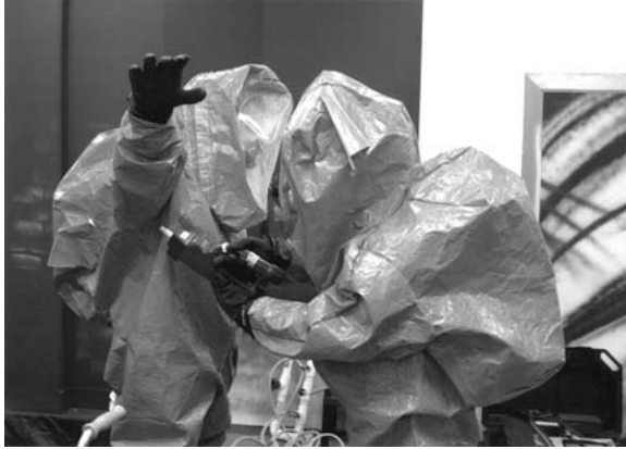
Figure 8.3 Hazmat technicians use an APD 2000 chemical agent monitor to detect chemical agents on Level A suit.
