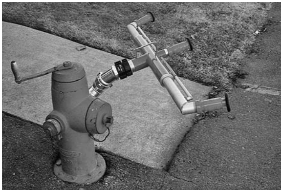
Figure 9.9 Trident/One Mass decontamination device that hooks onto a fire hydrant so an engine company is not tied up. Also works well for fixed facilities such as hospitals and chemical plants.
