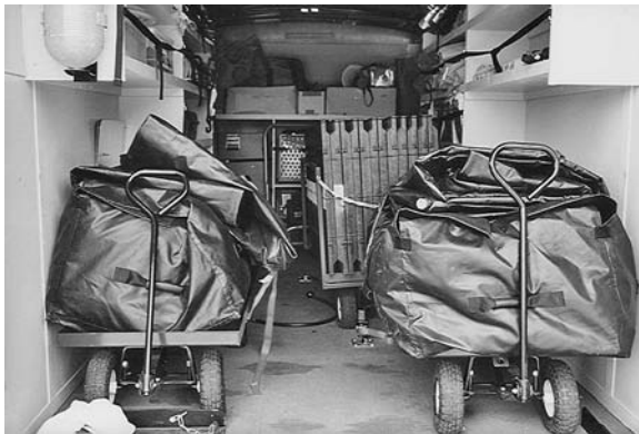
Figure 9.10 Portable mass decontamination tents on handdrawn carts for quick deployment.
