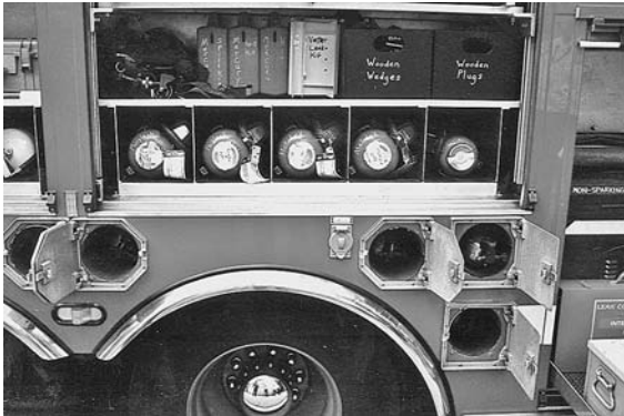
Figure 10.8 Spare air bottle compartments on Chicago Hazmat 512 using usually wasted space over the wheel wells.
