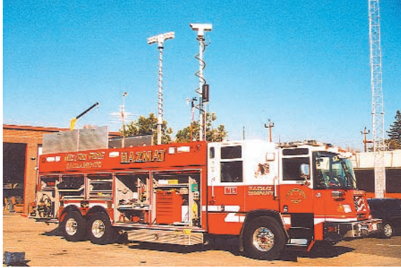
Figure 10.7 Sacramento County Fire Department's new hazmat unit with closed circuit television, complete analytical laboratory, light towers and other typical hazmat equipment.
