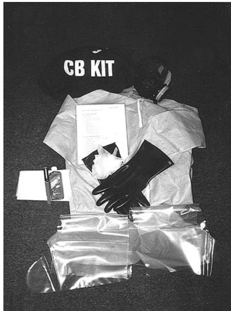
Figure 8.2 Chemical/biological (CB) personal protective equipment kits can be prepackaged for quick use by emergency responders when conducting on-scene testing of samples.
