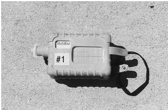
Figure 8.5 MultiRae Chemical Agent Monitor.
