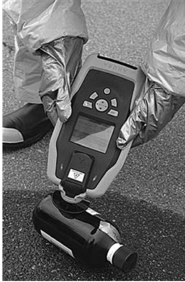
Figure 8.8 First Defender is ideal for identification of potentially hazardous materials directly through the container. (Courtesy AHURA Corporation, used with permission.)
