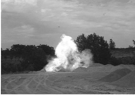
Figure 7.4 Flammable liquids ignited by explosives can produce overpressure damage, as well as set fires from the fireball.
