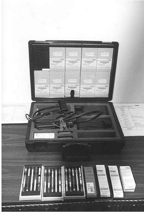
Figure 8.11 Draeger Civil Defense colorimetric tube kit for chemical agents.
