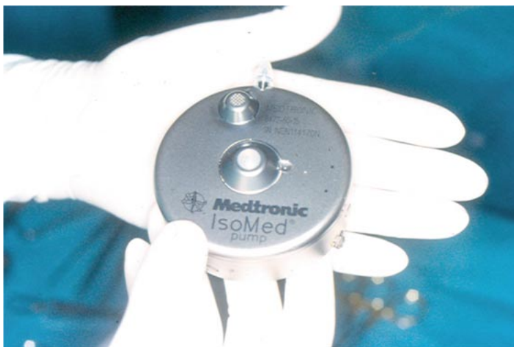
Fig. 2. Pump reservoir. Titanium box with two compartments – one for the artificial tear and the other is permanently filled with gas.
