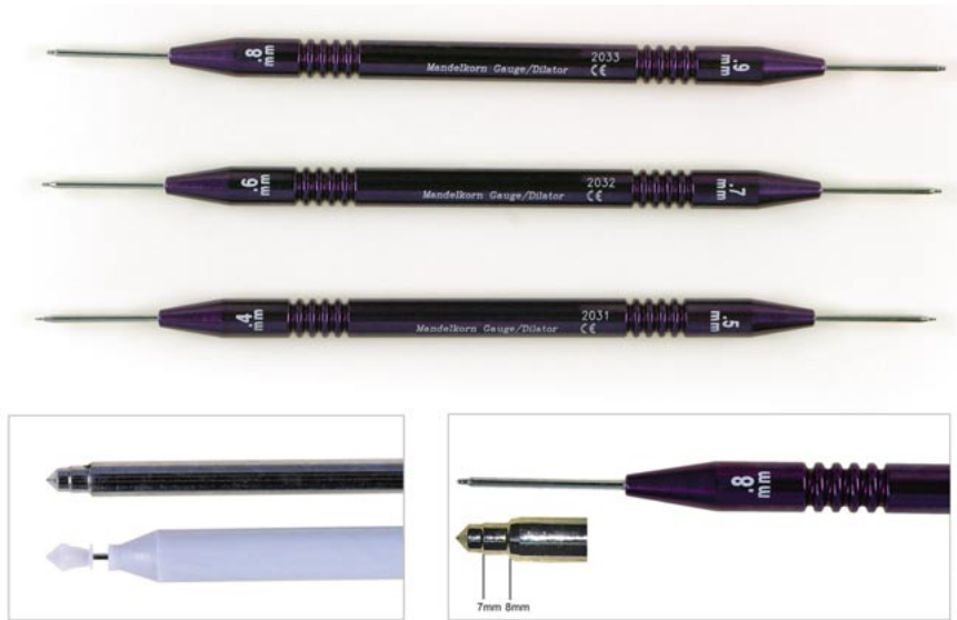
Fig. 2. Gauging system to measure the lacrimal puncta. The conical tip shows two steps. For the diameter indicated on the instrument the tip has to be fully inserted in the punctum. The first step equals a diameter of 0.1 mm lower than what is written on the instrument's handle.
