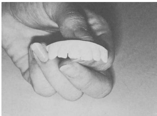
Fig. 8. Acrylic model of teeth for SEM examination.
