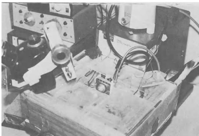
Figure 1. Modified Cryobox on LKB Microtome. There are several modifications shown here such as (1) increase in size (2) insulation both inside and out, (3) swingout binoculars, (4) multiple thermocouples with digital readout, (5) optic fiber lighting system, and (6) nitrogen gas line for cooling chamber.
