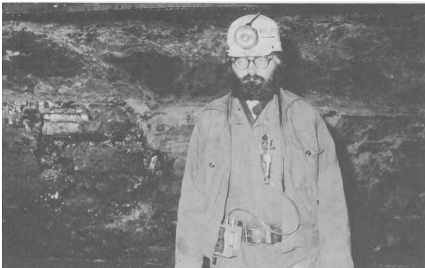
FIGURE 5. - Miner with collection filter cassette on jacket and pump unit on belt.
