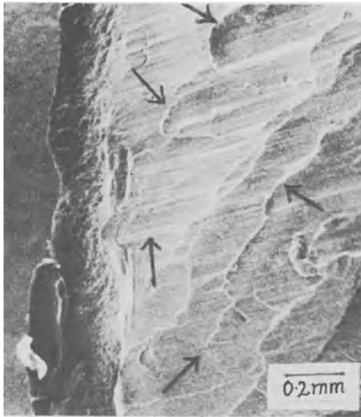
FIG. 7a. Surface of a cut end showing irregularities and fine striations.
