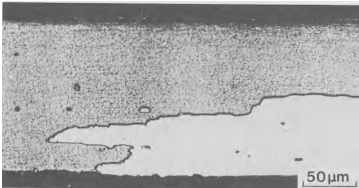
Fig. 2. Photomicrograph of same grade and size of tungsten wire as for fig. 1, annealed for 5 min. at 2700^\circ\text{C} ( 4892^\circ\text{F} ). Recrystallized microstructure; grains are "finger-locked". Etchant: Murakami (mod). Ref. (12). Reproduced with permission of American Society for Metals.
