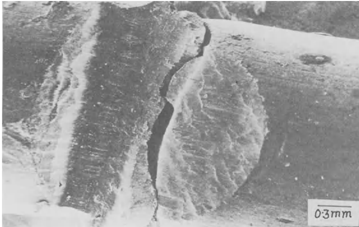
FIG. 5b. Corresponding fine striations on right cut end (Fig. 4)
