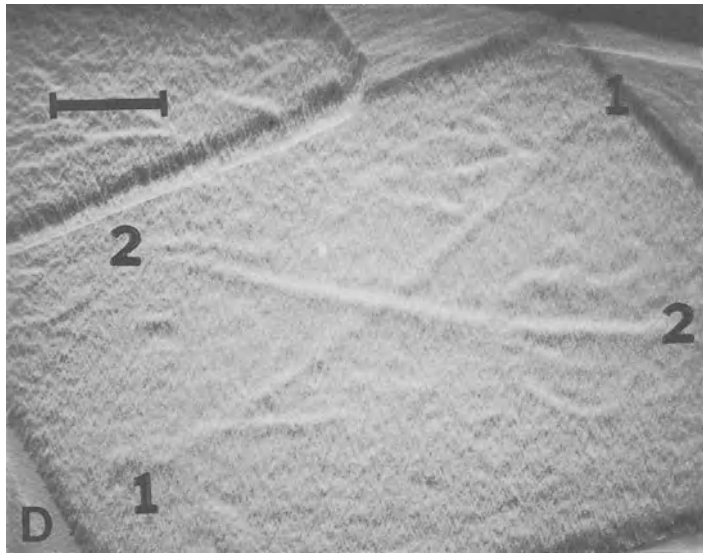
Fig. 2 BSE (C) and DMBS (D) images of a line crossing made with a soft pencil (Reliance ® , #2). The specimen in Fig. 2A and B was turned counter-clockwise until the lines 1 and 2 were inclined to the X, Y axes, as shown. See Fig. 2A and B for all other conditions. Bar: 1.0mm
