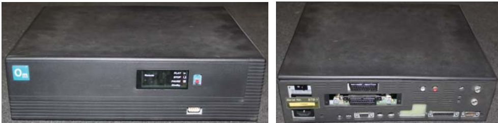
Figure 2.3 Arcon historic set-top box STB1 – first VoD system (Source: Reproduced by permission of Centre for Computing History, Cambridge, UK)
