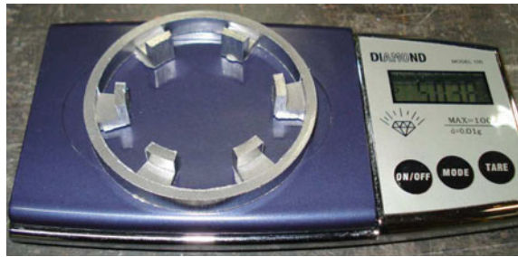
Fig. 4.8 a Molded stator of a PM claw-pole motor, and b FEM region of a pole of a stack
