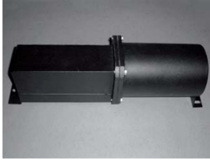
Figure 4. Neutron detector based on plastic scintillator and a photo multiplier
