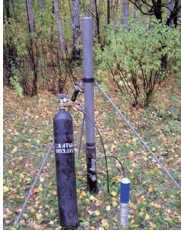
Figure 3. The pneumatic launching and dispersing unit for launching a container with chaff (tracers)
