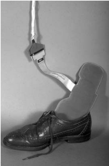
Figure 5.11. The insole for in-shoe measurement (Pedar-x System)
