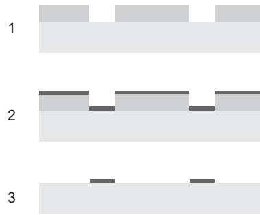
Figure 2.20: Lift off Process. 1. Patterning of a Sacrificial Layer. 2. Deposition of a Metal Film. 3. Remove Unwanted Metal Parts
