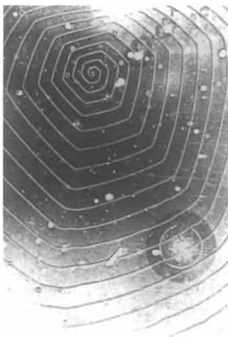
Figure 3.23. A growth spiral on a silicon carbide crystal, originating from the point of emergence of a screw dislocation (courtesy Prof. S. Amelinckx).
