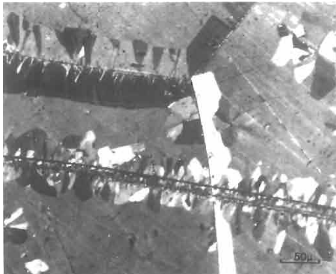
Figure 6.2. Stoichiometric CuPt, ordered at 550°C for 157 hours. Viewed under polarised light in reflection. Shows growth of ordered domains, heterogeneously nucleated at grain boundaries and surface scratches (after Irani and Cahn 1973).
