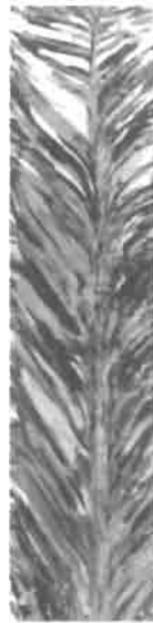
Figure 3.9. Macrostructure in an ingot.
