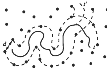
Figure 8.11. Reptation of a polymer chain. The chain moves snake-like through its confining virtual tube.
