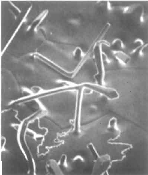
Figure 6.5. Whiskers grown at 1150°C on surface of an iron-aluminium alloy, imaged in an early scanning electron microscope \times 250 (Gardner and Cahn 1966).
