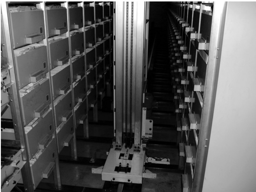
Fig. 6.19 A paper-based hospital archive with a robot system for storing and gathering boxes filled with patient records
