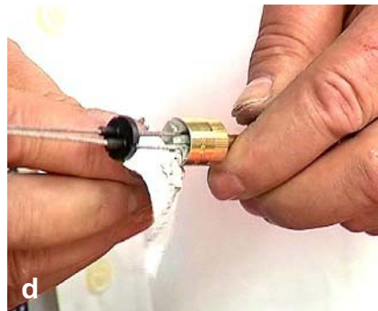
(c) Examine the inside of the pot for cleanliness and metallic hairs prior to filling with compound. (d) Overfilling the pot with compound. Use the plastic wrapping to prevent fingers coming into contact with the compound so as to ensure cleanliness of the seal.
