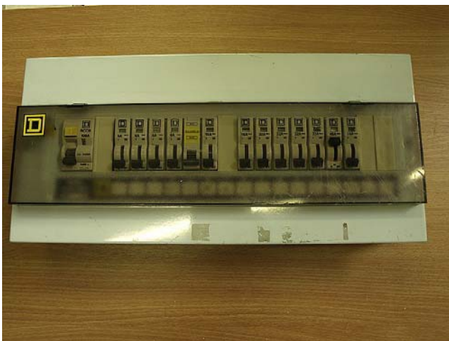
FIGURE 5.17 A 13-way consumer unit with final circuit MCBs and incorporating a 30mA RCD protective device.
