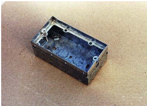
FIGURE 9.11 A metal conduit box with an extension piece for use where the depth has to be increased as building work progresses. See Fig. 9.9.
