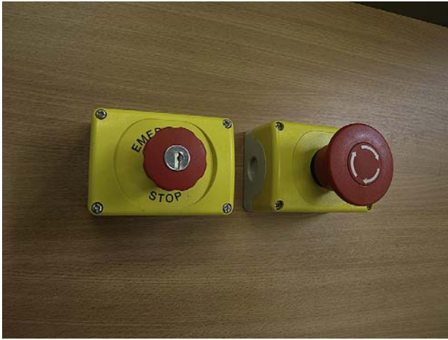
FIGURE 5.25 Emergency stop buttons, here shown with and without a key operated reset facility. The former (shown left) can be used where restoring the power must be carried out by authorised persons.
