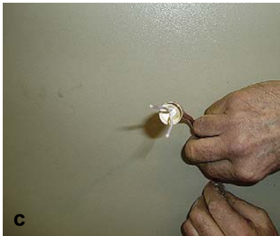
(c) Examine the inside of the pot for cleanliness and metallic hairs prior to filling with compound. (d) Overfilling the pot with compound. Use the plastic wrapping to prevent fingers coming into contact with the compound so as to ensure cleanliness of the seal.
