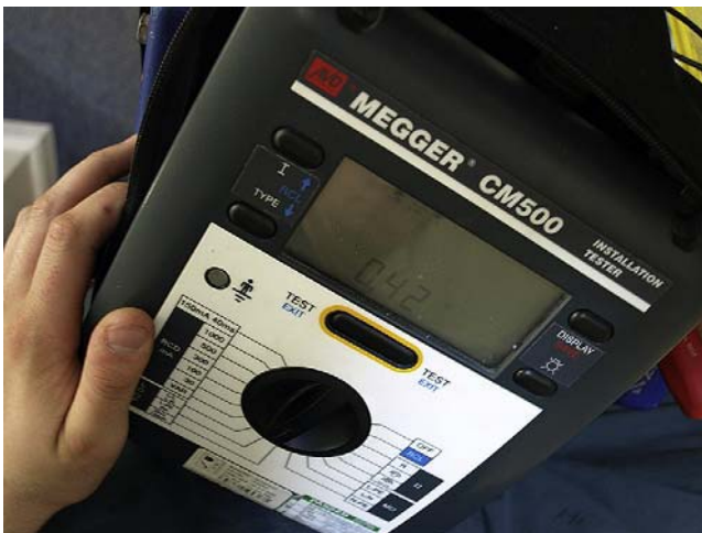
FIGURE 16.9 This digital instrument is capable of testing RCDs. Devices with ratings from 30mA to 1000mA may be tested.
