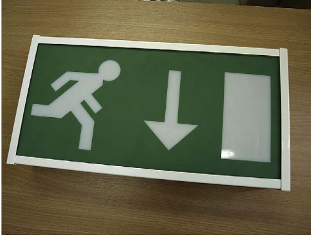
FIGURE 7.4 Automatic emergency lighting unit. The unit has a self-contained rechargeable battery, and control gear which detects mains failure and energises the emergency light.
