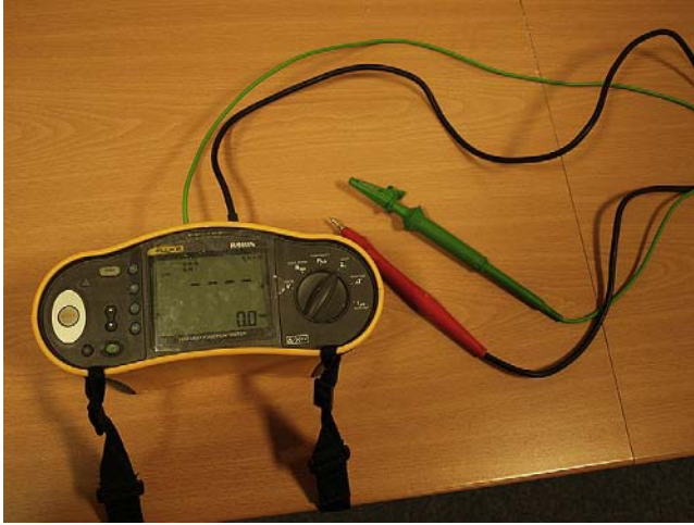
FIGURE 16.6 An instrument suitable for use as a digital loop tester is shown here. As with a number of instruments on the market, it will operate in several modes, easing the work of the tester.
