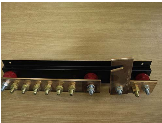
FIGURE 4.6 A main earth bar for use in a commercial installation. Note the link which is normally closed but can be unbolted for testing purposes.
