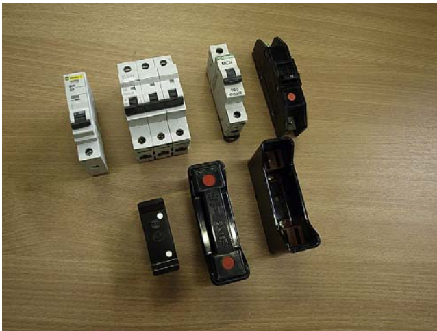
FIGURE 5.11 Overcurrent protective devices. Single- and three-phase MCB (top), a BS 1361 fuse (lower right) and rewirable fuses to BS 3036 (lower left). The use of HRC fuses or MCBs is strongly recommended.
