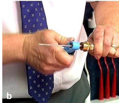
(a) A quick and accurate method of fitting the pot is by the use of a pot wrench. (b) Alternatively, a wrench can be used to fit the pot.
