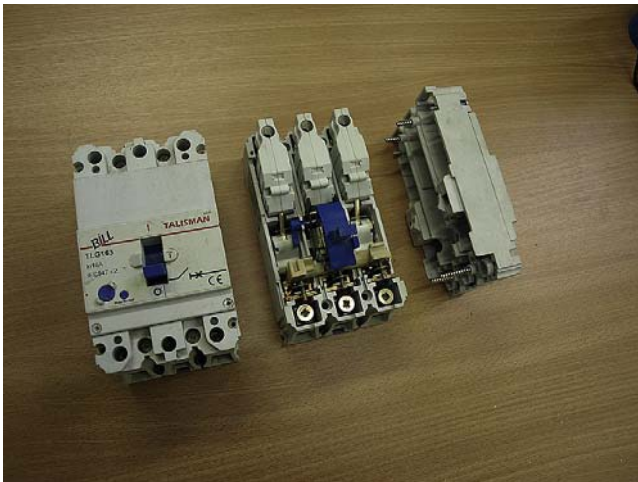
FIGURE 5.15 A view of an MCCB. This device incorporates both bimetallic and magnetic trip mechanisms to open the contacts under overload or short-circuit conditions. The operating toggle has three positions and shows when the breaker has tripped. A range of auxiliary components can be fitted such as undervoltage releases, or control interlocks. These MCCBs can be obtained with breaking capacities up to 150kA.
