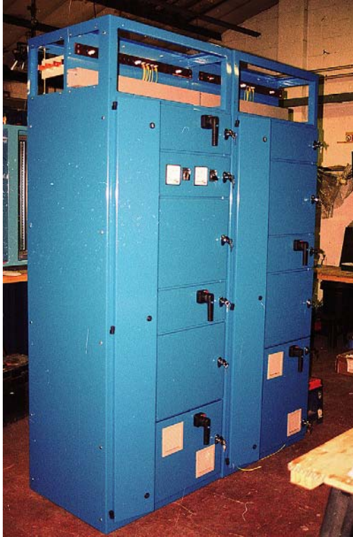
FIGURE 5.6 A protected switchboard with separate lockable compartments to house the incoming and outgoing cabling. Although these can be accessed from the front of the panel, it is still essential to allow space behind the panel to allow subsequent maintenance to be carried out at the rear (Pandelco Ltd).
