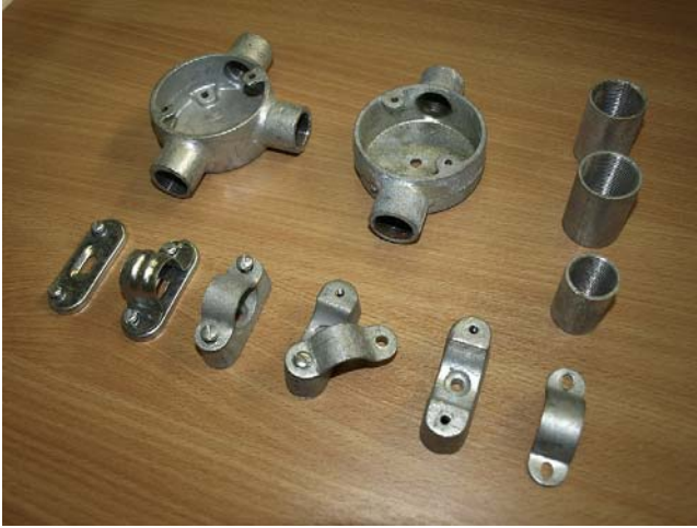
FIGURE 8.13 Screwed steel conduit is a widely used and very effective cable containment system. Conduit fittings such as these are readily available and a skilled electrician is able to present professional work using the equipment.
