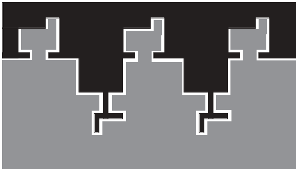
Fig. 7.13. Illustration of physical layout of fractal capacitors. Two terminals of these capacitors are represented with different shading.
