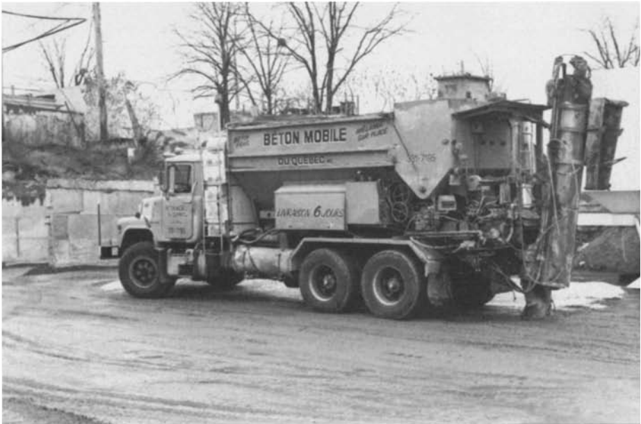
Figure 6.14 Typical concrete mobile truck.
