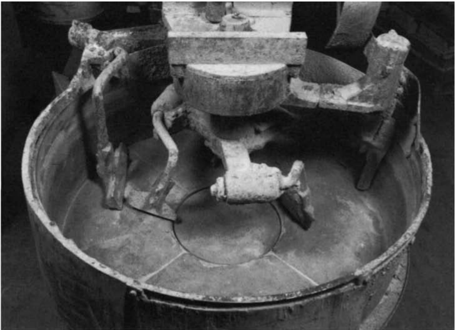
Figure 8.5 Typical concrete mixer used in the laboratory.
