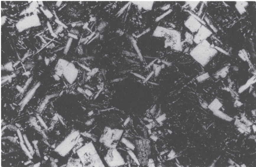
Fig. 6.39 Air-cooled or crystallized slag under polarized light in an optical microscope. The white prismatic crystals are melilite.
