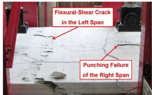
(b) Third bridge deck
