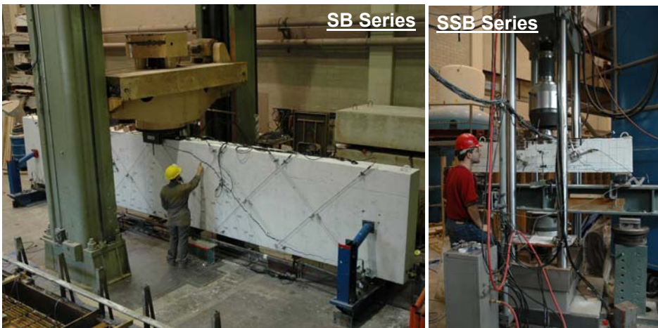
Figure 3: Specimen Test Setup
