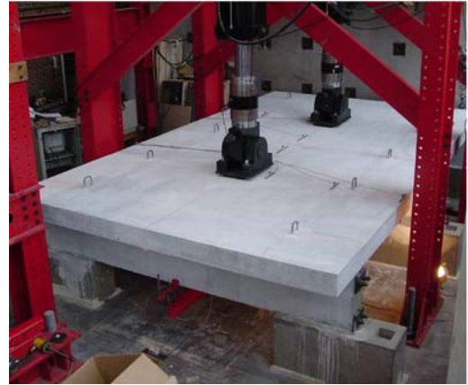
(b) First bridge deck prior to testing
