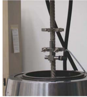
Fig 2. Elongation test apparatus.
