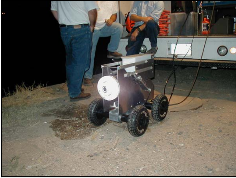
Figure 6. Second generation wheeled inspection robot with gpr
