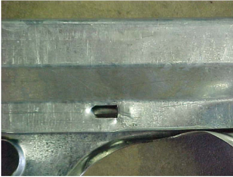
Fig. 5. Typical clinch failure.
