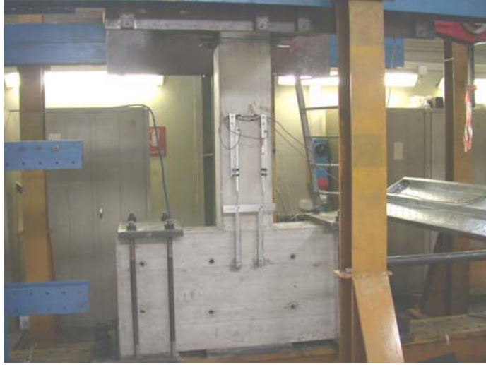
Fig. 12. Test rig and the column prototype.
