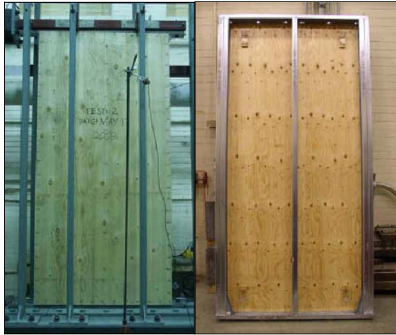
Figure 1. Typical 1220×2440 mm shear wall test specimens.
