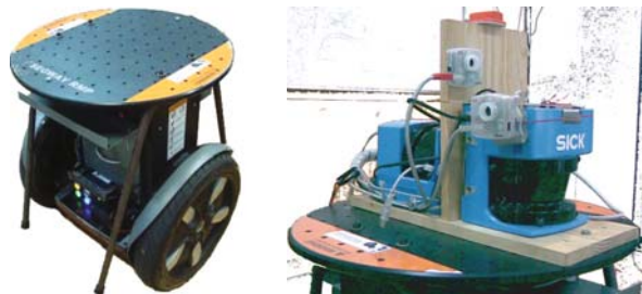
Fig. 7 The sensor platform comprising of two laser range finders and two cameras is mounted on the Segway RMP 200
