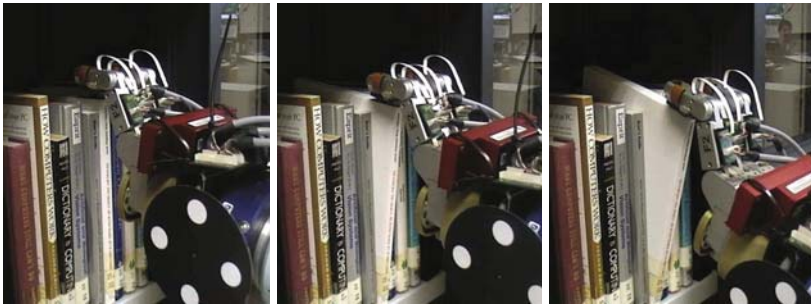
Fig. 6 The robot grasping the book by means of force and tactile-based continuous estimation of hand-to-object relative pose
