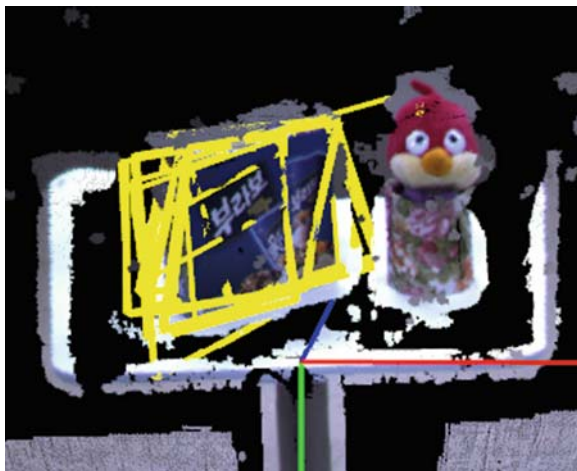
Fig. 8 Interpretation the rectangles based on perpendicular line pairs in set \Omega
