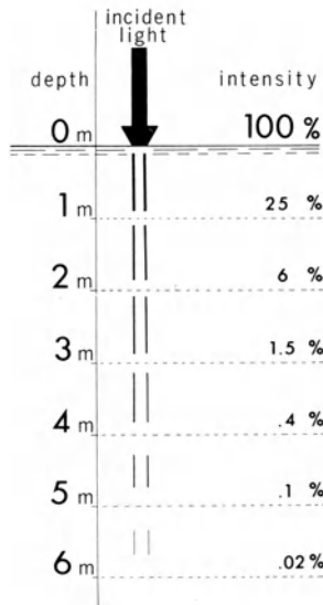
Fig. 10.6. Absorption of daylight in sea water follows an exponential law. With an increase of depth by 1 m, over 75 percent of the light is absorbed
