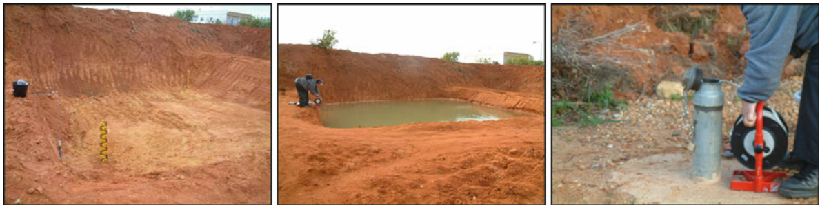
Fig. 10 Infiltration basin in the second layer and monitoring equipment used for the infiltration test
