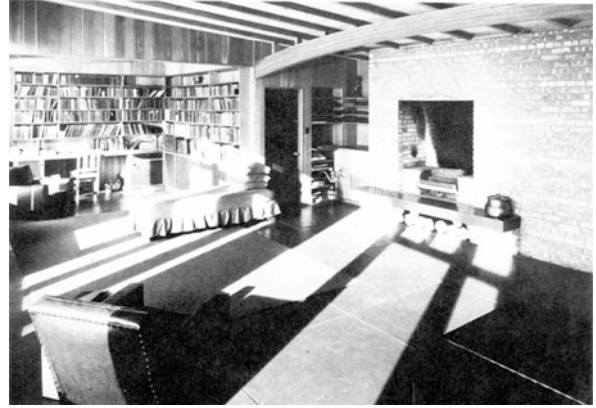
Passive Solar Heating in Built Environment. Figure 5 Direct gain maximized in the Duncan House (picture by permission of Pilkington, North America, Inc.)
