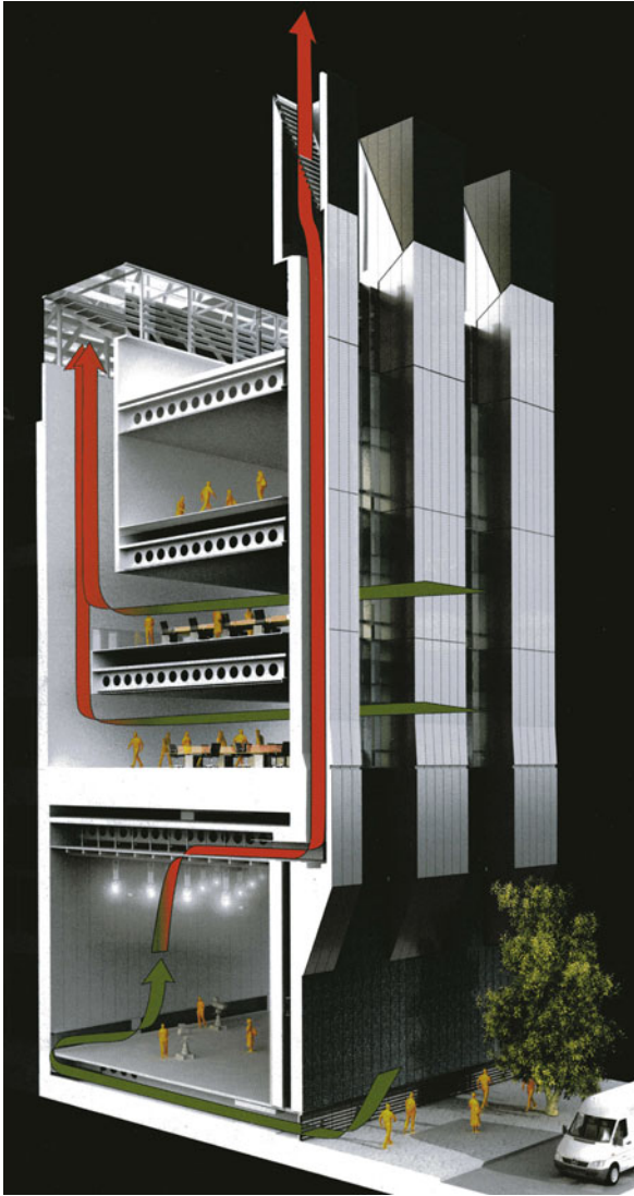
Natural Ventilation in Built Environment. Figure 33 Natural ventilation flow within the BSKyB television studios (Source: Arup Associates)
