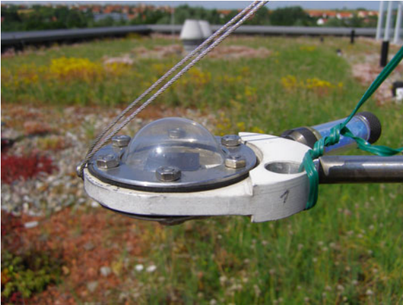
Green Roofs, Ecological Functions. Figure 6 Net Radio meter. Details from the research measurement facilities on a green roof at the University of Applied Sciences, Neubrandenburg, one of the Net – radiometers installed above different roof types to calculate the radiation balance
