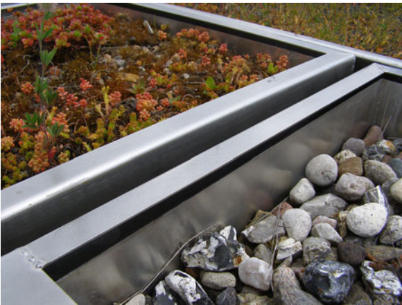
Green Roofs, Ecological Functions. Figure 7 Lysimeter. Detail of the roof lysimeter installation to measure the real water content of roof growing media and gravel roof
