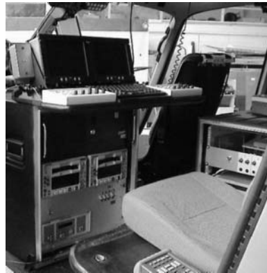
Helicopter interior showing LiDAR console
