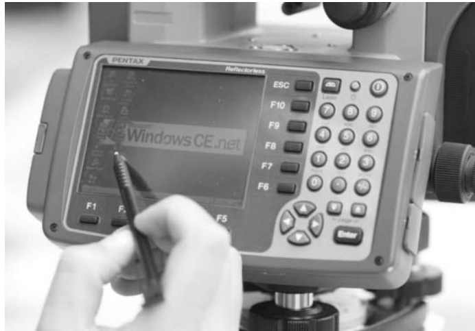
Figure 1.10 • Large graphics screen on total station (courtesy Pentax Industrial Instruments Co Ltd).
