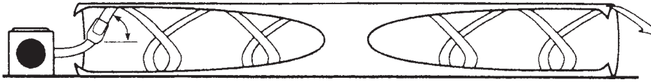
Figure 11.76 • A blower unit positioned to blow air into a pipe at a skew angle (courtesy Leica Geosystems.)
