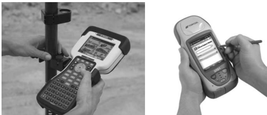
Figure 1.9 • Data collectors for surveying (courtesy Trimble & KOREC Group and Phoenix Surveying Equipment Ltd).
