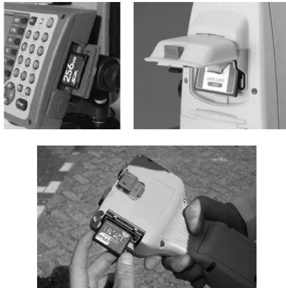
Figure 5.38 • Memory cards in total station and data collector (courtesy Pentax Industrial Instruments Co Ltd and Topcon).
