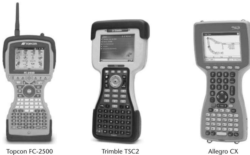
Figure 5.30 • Data collectors or controllers (courtesy Phoenix Surveying Equipment Ltd, Trimble & KOREC Group and Sokkia Topcon Co Ltd).
