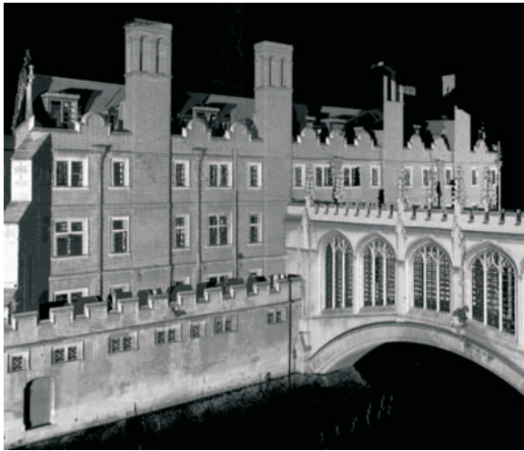
Figure 10.13 • Laser scan point cloud of the Bridge of Sighs, Cambridge (courtesy APR Services Ltd).
