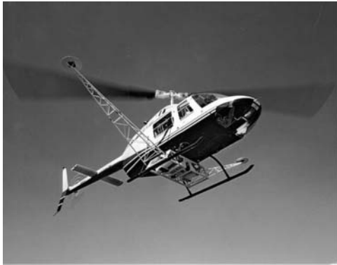
Helicopter with LiDAR head mounted underneath and video cameras on side booms
