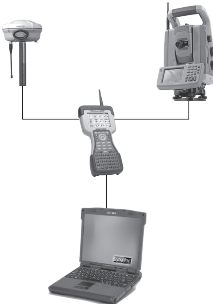
Figure 1.11 • Integrated surveying (courtesy Trimble & KOREC Group and General Dynamics Itronix).
