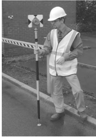
Figure 3.20 • Detail pole (courtesy York Survey Supply Centre).
