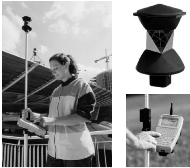
Leica TPS1200 pole-mounted 360° prism and controller (uses radio communication to total station)
