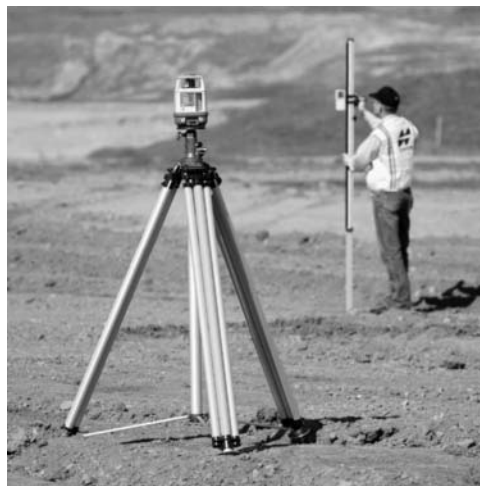
Figure 11.80 • A rotating laser in use with its sensor (courtesy Topcon).
