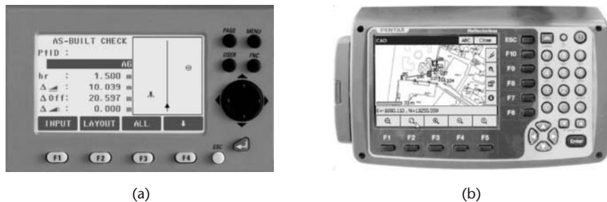
Figure 5.21 • Examples of total station keyboards and displays: (a) Leica FlexLine TS02 with basic functions required on site; (b) Pentax W-800 with greater functionality required for mapping and other surveys (courtesy Leica Geosystems and Pentax Industrial Instruments Co Ltd).
