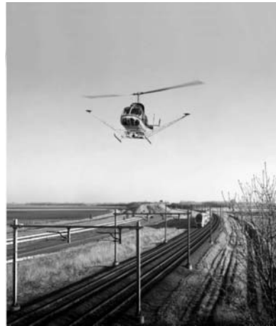
LiDAR survey of railway
