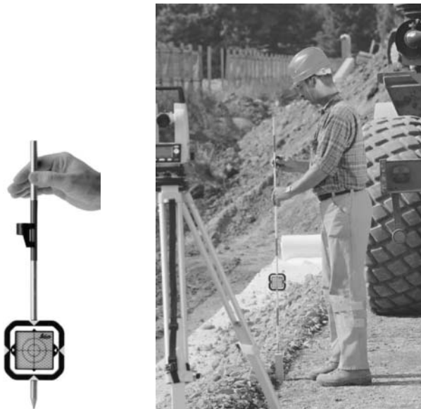
Figure 5.17 • Pole-mounted plastic reflector (courtesy Leica Geosystems).
