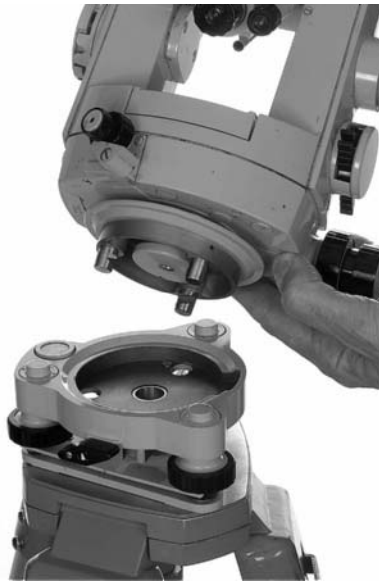
Figure 3.4 • Detaching theodolite and tribrach.
