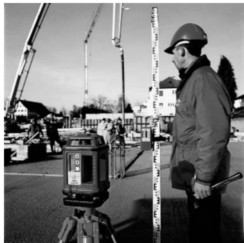
Figure 11.81 • Rotating laser sensor fitted to a levelling staff (courtesy Leica Geosystems).
