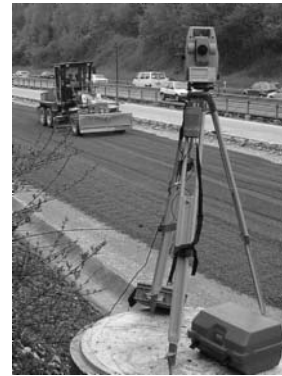
Figure 11.90 • A 360° prism mounted on a grader for machine control with a total station (courtesy Leica Geosystems).
