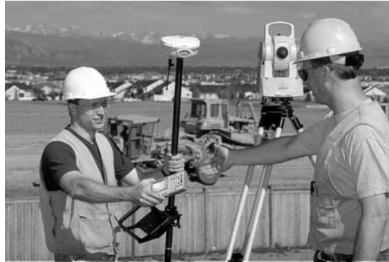
Figure 5.34 • Exchange of control unit from GNSS receiver to total station (courtesy Trimble & KOREC Group).
