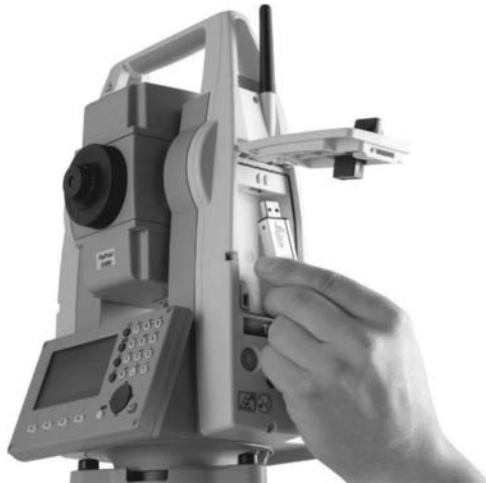
Figure 5.40 • Data transfer with USB stick (courtesy Leica Geosystems).
