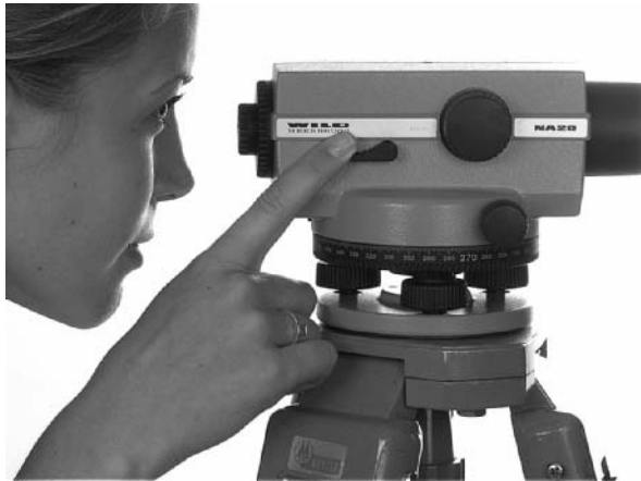
Figure 2.14 • Compensator check (courtesy Leica Geosystems).
