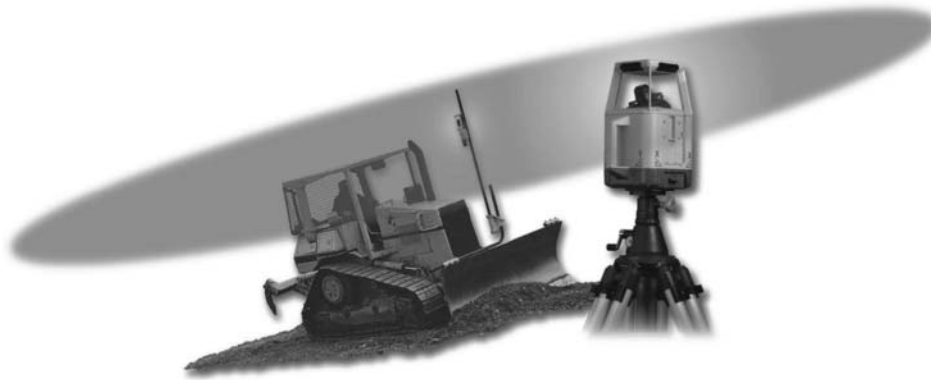
Figure 11.97 • Principle of laser controlled grading (courtesy Topcon).
