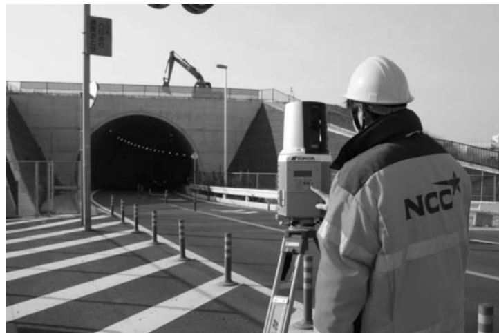
Figure 10.12 • A laser scanner in operation (courtesy Topcon).
