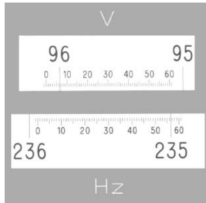
Vertical circle reading 96^{\circ}06.5' Horizontal circle reading 235^{\circ}56.4'
