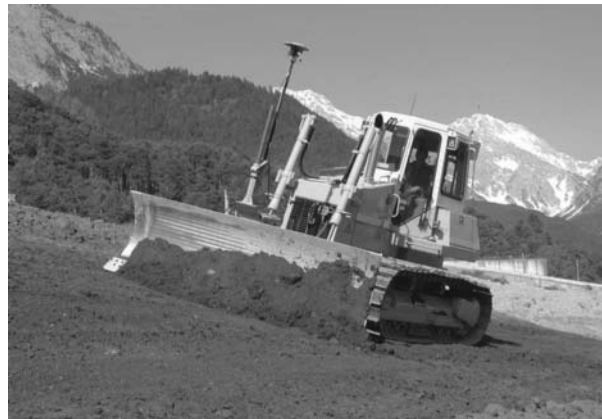
Figure 11.92 • GNSS antenna mounted on a dozer blade (courtesy Topcon).
