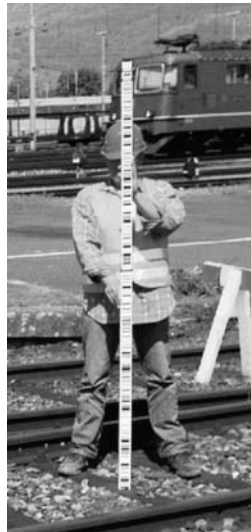
Figure 2.18 • Bar-coded levelling staff (courtesy Leica Geosystems).
