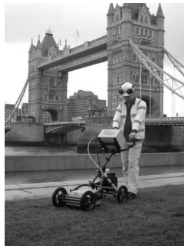
Figure 10.30 • A GPR instrument in operation (courtesy Subscan Technology Ltd.).
