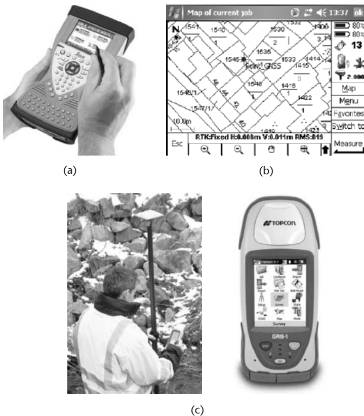
Figure 10.8 • Graphical data collection and editing for detail surveying by GNSS. (a) Leica CS15 Viva Controller (courtesy Leica Geosystems); (b) Trimble R7 GNSS receiver screen display (courtesy Trimble & KOREC Group); (c) Topcon GRS-1 (courtesy Phoenix Surveying Equipment Ltd).
