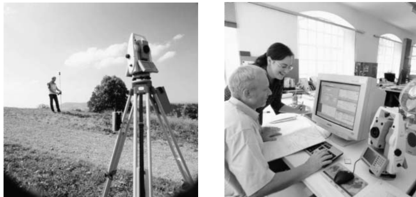
Figure 1.6 ● Detail survey by total station with computer processing (courtesy Leica Geosystems).
