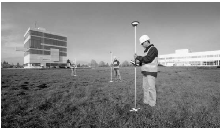
Figure 10.7 • Detail surveying using a GNSS receiver (courtesy Leica Geo-systems).
