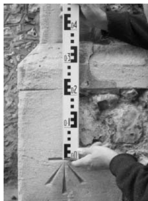
Figure 2.3 • Ordnance Survey Bench Mark (part reproduced by permission of Ordnance Survey on behalf of the Controller of Her Majesty's Stationery Office, © Crown Copyright 100024463).
