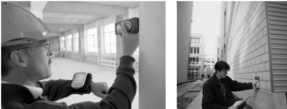
Figure 5.27 • Leica DISTO hand-held laser distance meter in use (courtesy Leica Geosystems).
