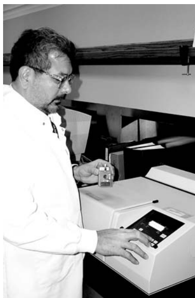
Dave Segura prepares to use an FTIR instrument for simethicone analysis. Notice the liquid sampling cell in Dave's left hand.
