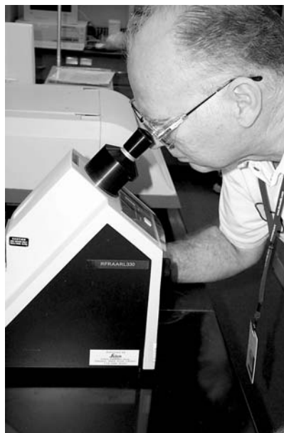
John Hannon, an analyst for a pharmaceutical company, uses a refractometer for the determination of the quality of flavor oil used in cough medicine preparations.
