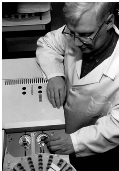
Richard Mathias makes adjustments on the auto-sampler attached to a gas chromatograph at the Midwest Research Institute.
