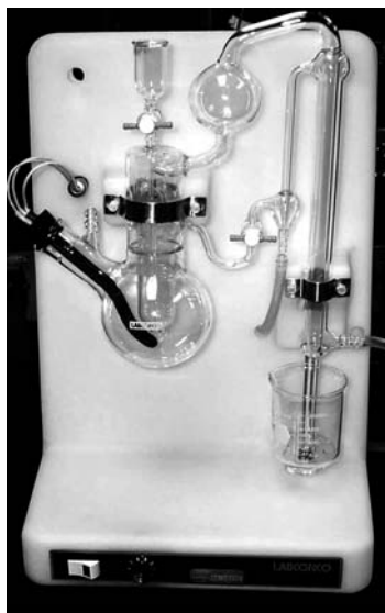
FIGURE 5.13 A photograph of a commercial Kjeldahl distillation unit. The heating chamber (with heating element) is in the left center, the baffle in the top center, the condenser in the right center, and the beaker (receiving vessel) for holding the standard acid solution in the lower right.
