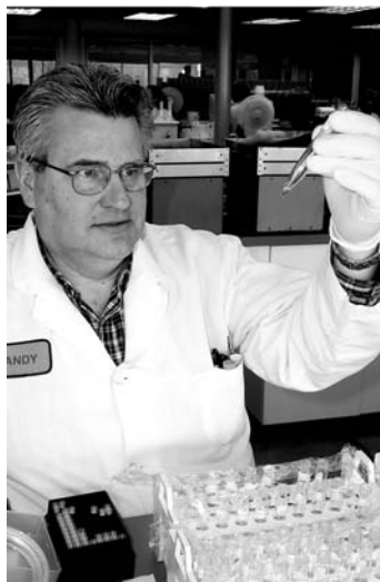
Randy Karl of MDS Pharma Services in Lincoln, Nebraska, examines a centrifuge tube containing a heparinized plasma sample prior to performing an extraction procedure using ethyl acetate.
