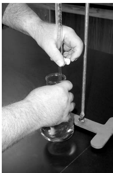
FIGURE 4.15 The correct way for a right-handed person to position his or her hands when performing a titration.
