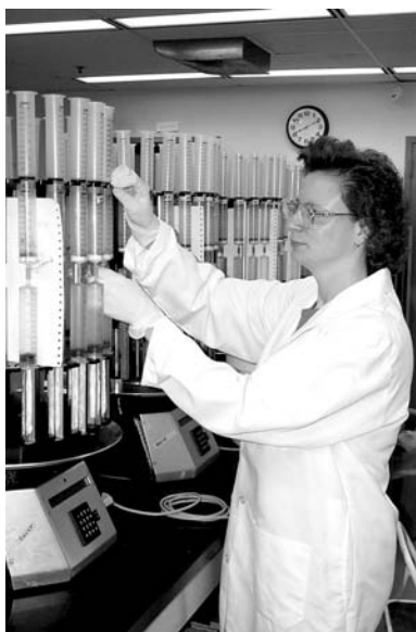
Patty Jones checks the operation of an automatic mechanical vacuum extractor in the chemistry section of the Natural Resources Conservation Service (NRCS) Soil Survey Laboratory in Lincoln, Nebraska.
