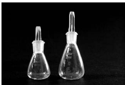
FIGURE 15.15 Two glass pycnometers. The capacity of the one on the left is 5 mL. The capacity of the one on the right is 10 mL.
