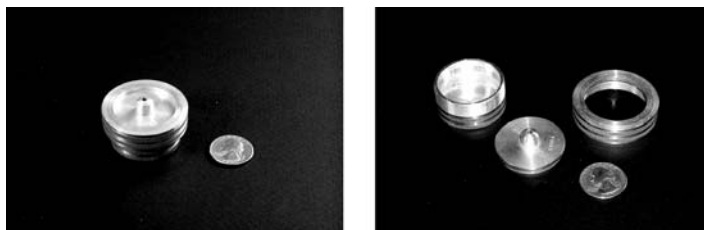
FIGURE 15.16 An aluminum pycnometer assembled (left) and disassembled (right). The quarter in the photos is to indicate the size of the pycnometer.
