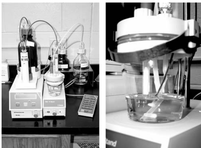
FIGURE 14.14 Photographs of a typical volumetric unit. The complete unit is shown on the left and a close-up of the titration vessel on the right. The dual platinum wire probe is visible in the right photograph as is the tube (dark in color) that introduces the titrant to the solution.
