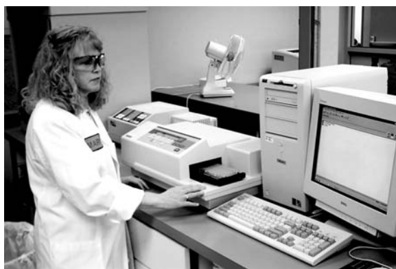
Mary Peterson of MDS Pharma Services in Lincoln, Nebraska, prepares to insert a 96-well plate into the UV-VIS scanner used to detect antibodies that have been bound to a seed drug.
