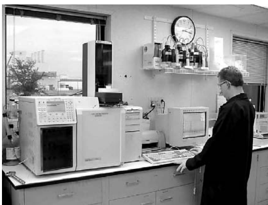
Reagan Boles of SACHEM Inc. measures organic impurities in ultrapure solvent products at the parts per million level using gas chromatography.
