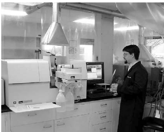
Robert Krause of SACHEM Inc. analyzes trace elements in ultrapure chemical products at the sub-parts per billion level using graphite furnace AA spectrophotometry.
