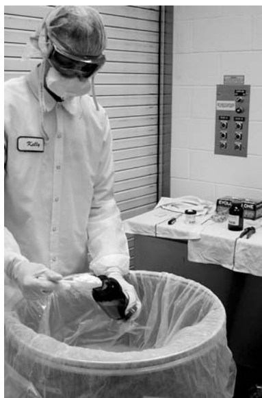
Kelly White, pharmaceutical sampling technician, takes a sample of magnesium hydroxide from a drum of this strong base. Notice the extraordinary personal protective equipment and contamination protection.
