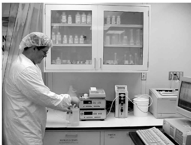
Paul Plumb of SACHEM Inc. counts particles in the ultrapure solutions of TMAH by a laser-equipped particle counter in the clean room. Notice the hair net and special lab coat.
