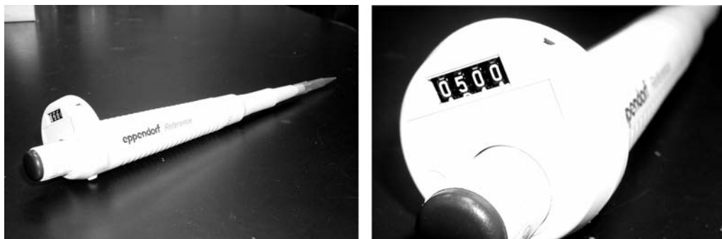
FIGURE 4.17 A typical commercial pipetting device. The close-up on the right shows that it is “dialed in” to deliver 500 \mu\text{L} , or 0.5 mL.
