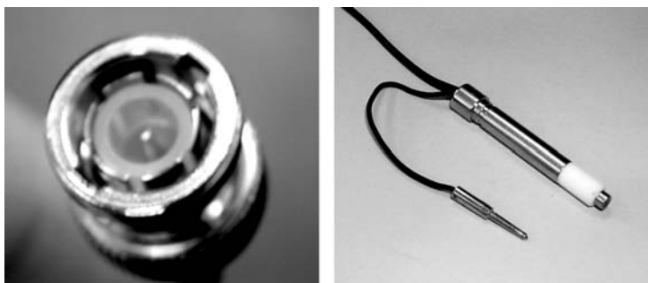
FIGURE 14.9 Photographs of the electrical connections to the combination pH electrode. Left, the bnc type of connection. Right, two separate connections to be made to the pH meter.
