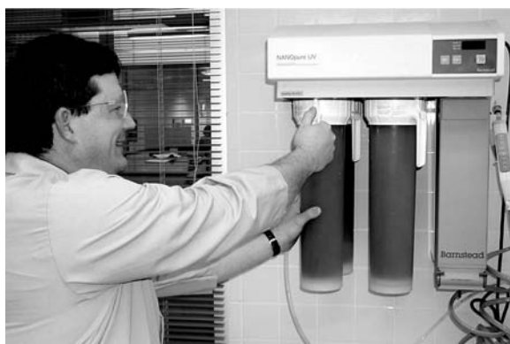
Eric Lee of the City of Lincoln, Nebraska, Water Treatment Plant Laboratory prepares to replace a spent deionization cartridge with a new one.
