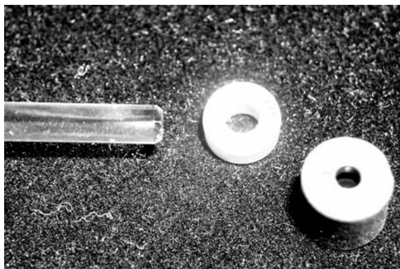
FIGURE 13.5 A photograph showing a pump piston (left), a pump seal (center), and a check valve (right). The pump seal is made to fit snugly over the piston, which is approximately 1/4 in. in diameter.
