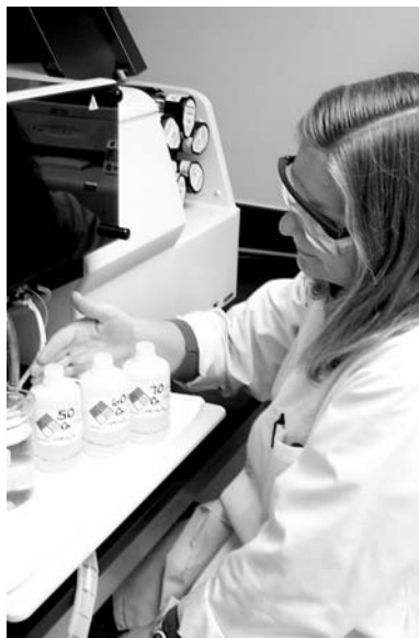
Cindy Wiebeck of the Nebraska State Agriculture Laboratory aspirates calcium standards into the atomic absorption flame in order to calibrate the instrument for the analysis of fertilizer for calcium. In the background, note the hollow cathode lamps held in a rotating turret in the instrument.
