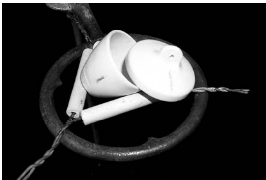
FIGURE 3.9 A crucible tilted to one side, with lid partially covering the opening. This allows the burner flame to be directed to the bottom of the crucible and air to circulate into the crucible.
