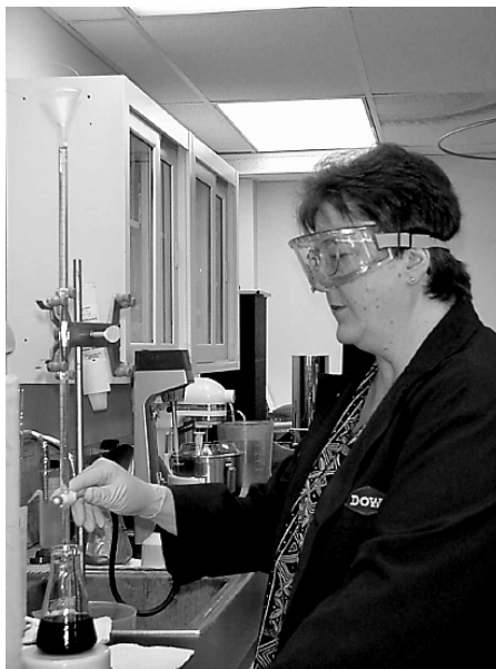
Pamela Slavings of the Dow Chemical Company in Midland, Michigan, performs the peroxide titration.
