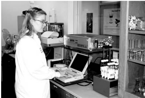
Jessica Weinland, a laboratory technician for a pharmaceutical company, operates a TOC analyzer to monitor the organic contaminants in the water used in preparing pharmaceutical formulations.
