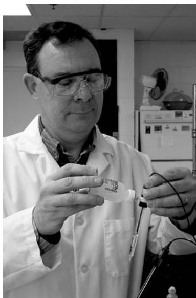
Charlie Focht of the Nebraska State Agriculture Laboratory refills a saturated calomel electrode with saturated potassium chloride while preparing to analyze animal feed samples for sodium chloride via a potentiometric titration.
