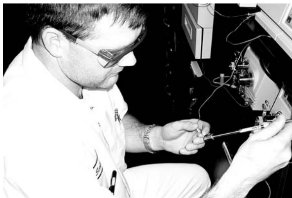
Scott Jenkins, a pharmaceutical analyst, changes HPLC columns in preparation for analyzing for a different analyte in a different pharmaceutical preparation.
