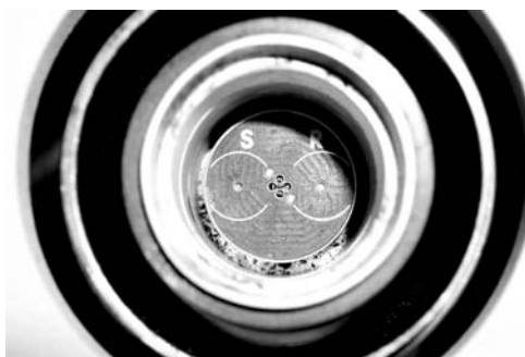
FIGURE 15.10 A photograph of the interior of a small oven used for differential scanning calorimetry. The crucibles for the sample (S) and reference material (R) are placed in the small circles.
