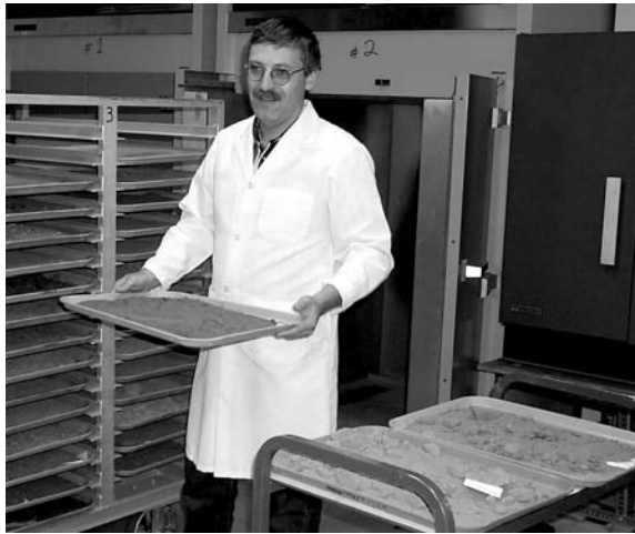
Larry Arnold, a technician with the National Soil Survey Laboratory in Lincoln, Nebraska, prepares soil samples for particle size analysis.
