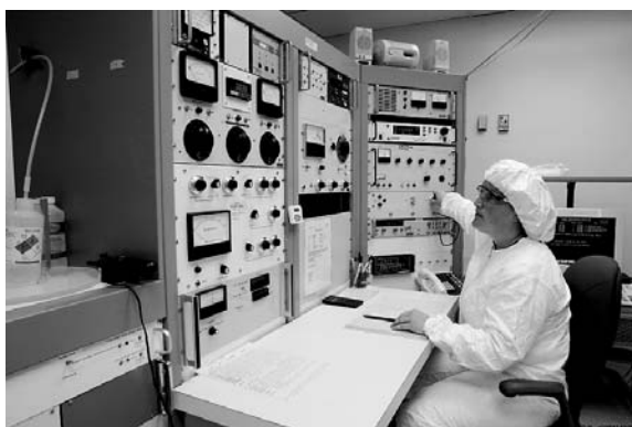
Kim Israel, a technician at LANL, Chemistry Division Bioassay Program, runs a thermal ionization mass spectrometry (TIMS) instrument.
