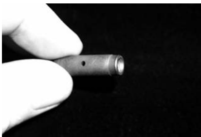
FIGURE 9.13 The small graphite cylinder that is the graphite furnace. The small hole is for introducing samples to the interior of the cylinder.
