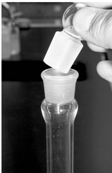
FIGURE 4.6 A tapered ground glass stopper may be used with a flask with a ground glass opening. A tapered plastic stopper may also be used.
