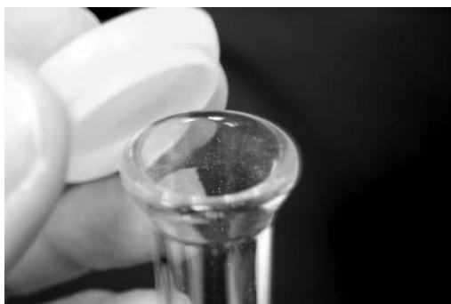
FIGURE 4.7 Left, the top of a volumetric flask designed for a snap cap. Right, the imprint on the base of the flask indicating the size of snap cap required (#5).
