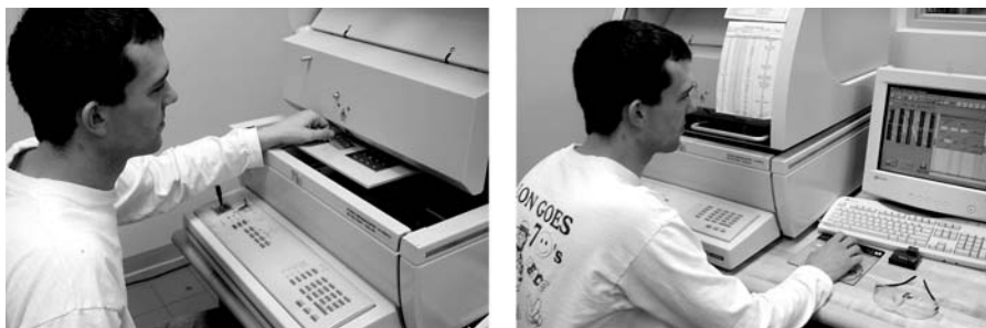
Troy Heany of the Molex, Inc., positions an electroplated specimen in the x-ray diffractometer (left) and then observes the computer image of the location on the specimen where the thickness is measured (right).
