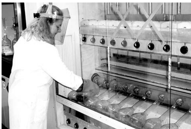
Cindy Wagner-Wiebeck sets a Kjeldahl flask in place in a fume hood dedicated to Kjeldahl sample digestion.
