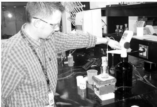
Clayton Allsman, a laboratory technician for Molex, Inc., titrates a plating bath sample for acid content using an automatic bottle-top buret.
