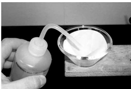
FIGURE 3.8 Rinsing the precipitate and filter paper with distilled water from a squeeze bottle.
