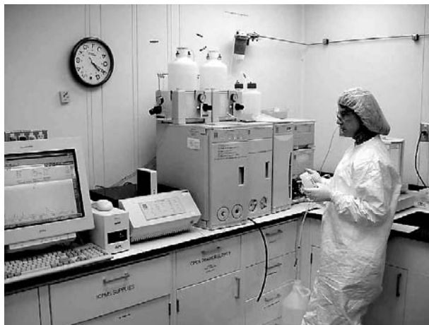
Kay Lones of SACHEM Inc. conducts analyses for trace anions in ultrapure TMAH products at the parts per billion level by using ion chromatography in a clean room like that described in Workplace Scene 1.2.
