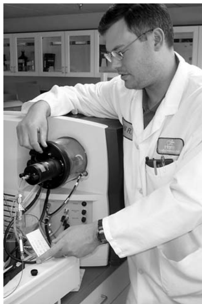
Jon Rathe, a technician in the LC-MS laboratory at MDS Pharma Services, checks out the thermospray interface on one of the LC-MS units in this laboratory.
