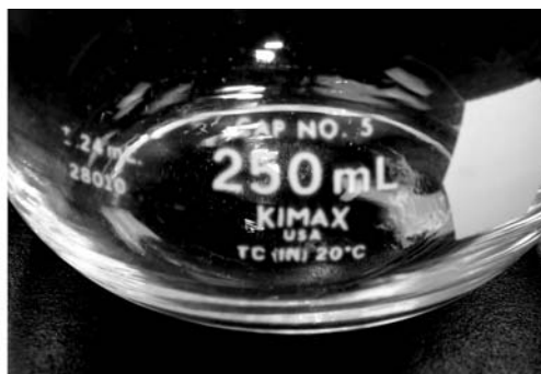
FIGURE 4.7 Left, the top of a volumetric flask designed for a snap cap. Right, the imprint on the base of the flask indicating the size of snap cap required (#5).
