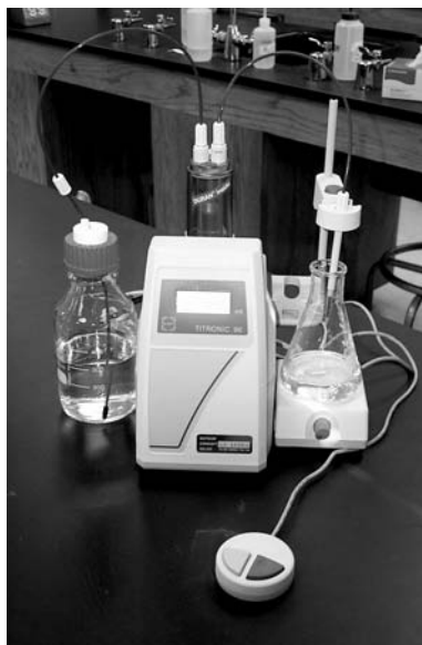
FIGURE 4.18 An automatic titrator. A pump draws the titrant from the reagent bottle on the left and fills the reservoir in the back of the unit. Pressing a key on the keypad in the foreground delivers titrant to the titration flask on the right as the solution is automatically stirred. The volume delivered is displayed on a digital readout.
