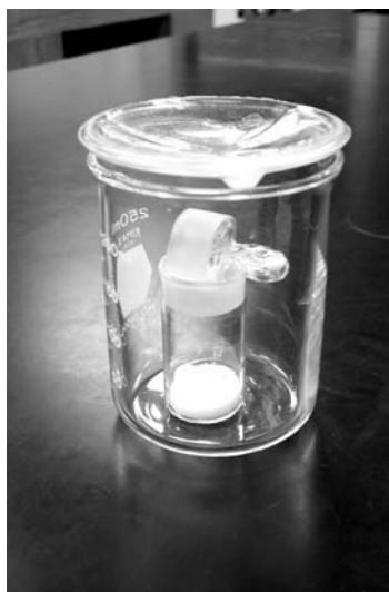
FIGURE 3.6 A weighing bottle with sample, lid ajar, in small beaker, ready to be placed in a drying oven for the purpose of drying the contained sample.
