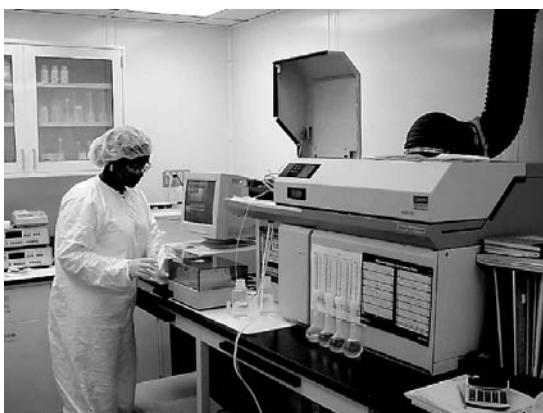
Katrice Harris of SACHEM Inc. measures trace elements in ultrapure TMAH solutions at the parts per thousand level by using ICP-MS in a clean room.
