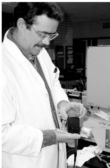
Steve Kruse of the City of Lincoln, Nebraska, Wastewater Treatment Plant Laboratory examines a faulty detector module taken from the flow injection analysis system in use in the laboratory.
