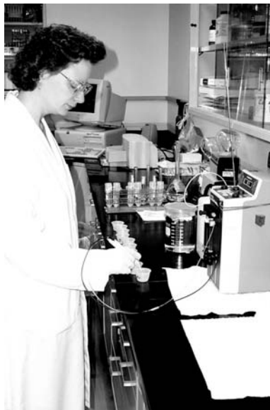
Patty Jones, a physical science technician at the NRCS Soil Survey Laboratory, prepares extracts for phosphorus analysis using a diluting device.
