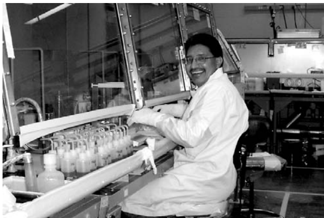
Elmer Lujan, a technician with the Los Alamos National Laboratory in New Mexico, prepares metal samples to be analyzed for plutonium using controlled-potential coulometry. (Photo by Laurie Walker.)
