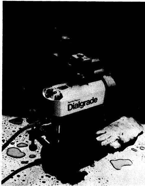
Figure 14.46 Pipelaying laser (courtesy Spectra-Physics Ltd)
