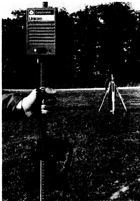
Figure 4.25 Communication system (courtesy Geotronics (UK) Ltd)
