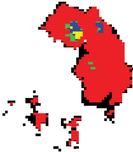
Figure 4.18 Pullout load and active filament curves during pullout, along with the colored images of the active fibers, for bundled yarn glass systems exhibiting brittle behavior (a), and ductile telescopic failure (b). (Bentur et al., 2010; Yardimci et al., 2011), using the FILT test method developed by Banholzer et al. (2006). (Continued)
