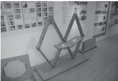
Figure 11.2 Development of honeycomb structural elements for axial and shear resistance as well as free-form interlacing structural triangular elements.
