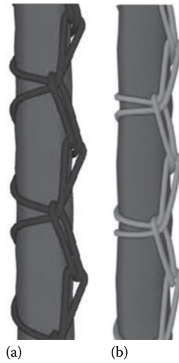
Figure 4.73 Simulated pillar stitch around a multifilament bundle: (a) close stitch and (b) open stitch. (After Dolatabadi, M.K. et al., Mater. Struct. , 44, 245, 2011.)
