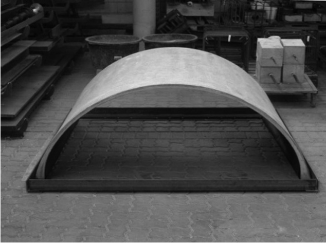
Figure 3.4 Thin, curved barrel shell made of TRC for roof construction. (From Hegger, J. and Voss, S., Eng. Struct. , 30, 2050, 2008.)
