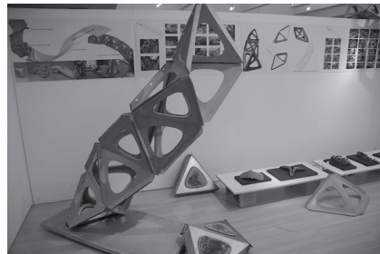
Figure 11.2 Development of honeycomb structural elements for axial and shear resistance as well as free-form interlacing structural triangular elements.
