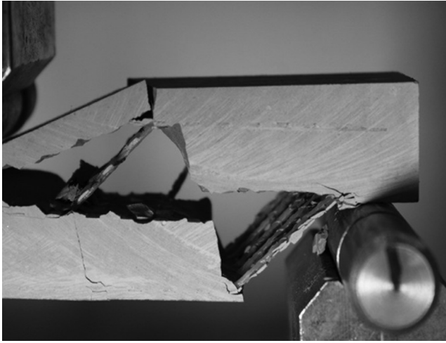
Figure 5.68 Delamination of 2D fabric composite with two fabric layers tested in bending. (From Adiel Sasi, E. and Peled, A., Composites , 74, 153, 2015.)
