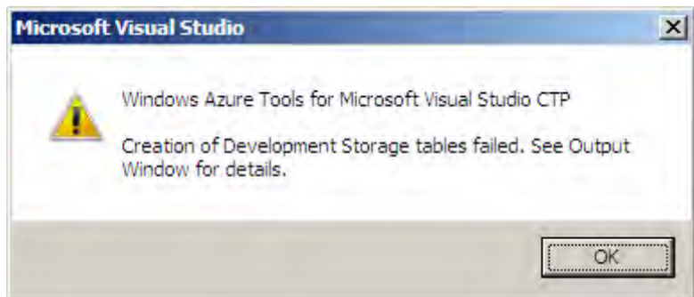
Figure 1-13. Error message from the compiler when attempting to regenerate the storage tables if a non-portable data type is added to a cloud table
