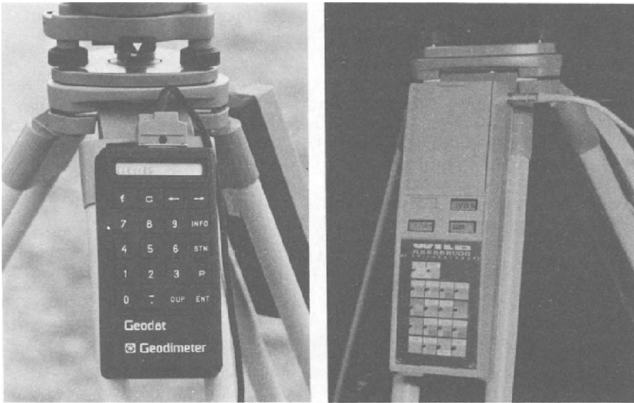
Figure 4.28 Data storage or recording units (courtesy Geotronics (UK) Ltd and Wild Heerbrugg (UK) Ltd)
