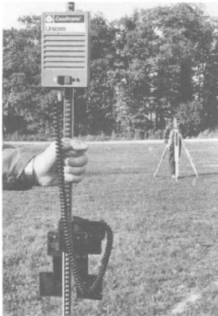
Figure 4.25 Communication system (courtesy Geotronics (UK) Ltd)
