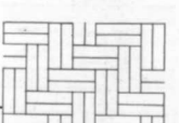
23 Heavily loaded floor finish with bricks on edge (herringbone pattern as in parquet)
