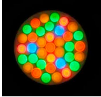
Figure 14.15 2W LED lamps give the same light output as 25W filament lightbulbs.
