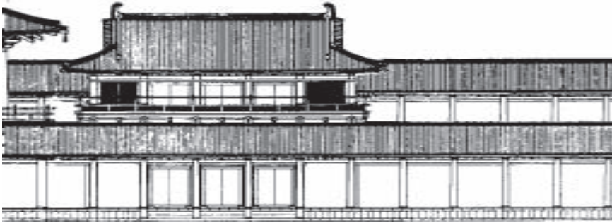
Fig 3.3 Daigokuden (Imperial Audience Hall) of Nara Palace. Front elevation of the main hall and flanking towers as seen from the south. The Komon and enclosing cloisters are situated at the front. Reconstruction drawing by the Nara National Cultural Properties Research Institute (Source: Nara National Cultural Properties Research Institute)
