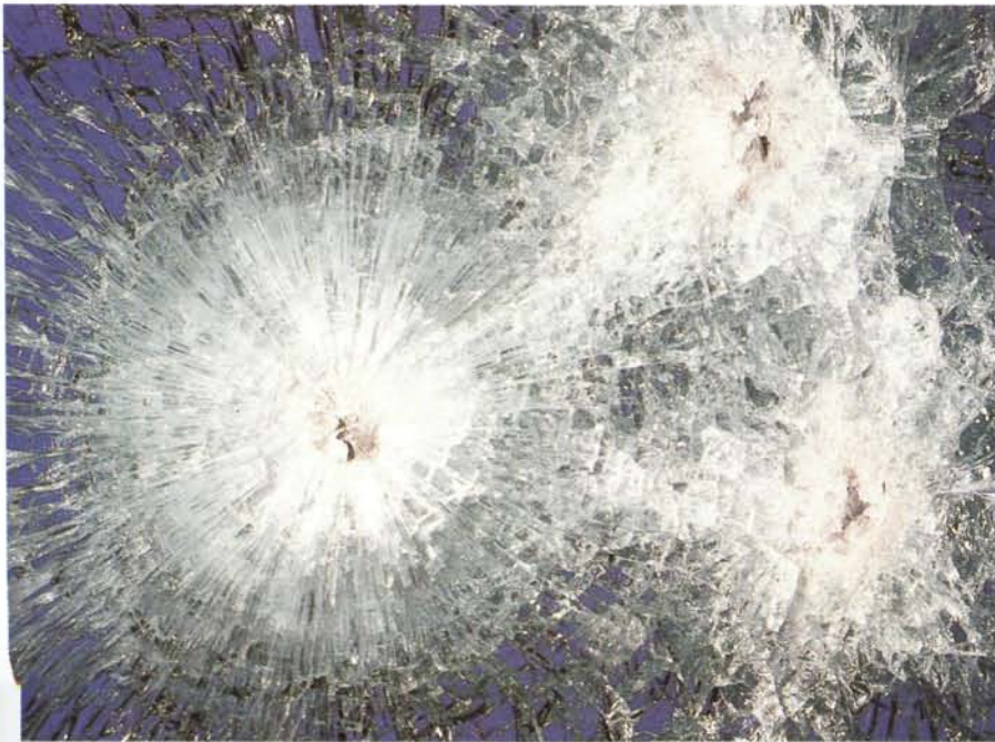
Fig. 2.10 Laminate damaged by bullet (WB & B Strategic communications)
