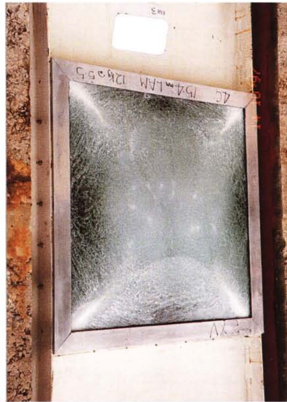
Fig. 15.4 Laminated glass panel after being blast tested (courtesy of Security Facilities Executive)
