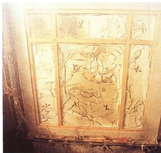
Fig. 2.20 An intumescent interlayer (left) before and (right) after it has done its job (courtesy of Pilkington)
