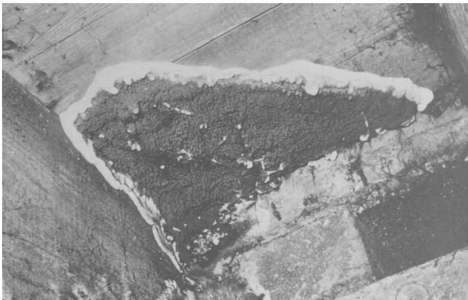
Figure 30 Dry rot fruiting body ( Crown copyright: Reproduced by permission of the BRE Princes Risborough Laboratory )
