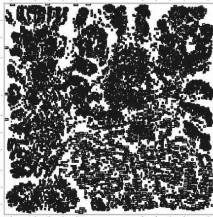
Fig. 10.11. Global placement on a testcase (#cells = 12506) with utilization = 0.4. The half-perimeter wirelength is 2.2024 \times 10^6 .
