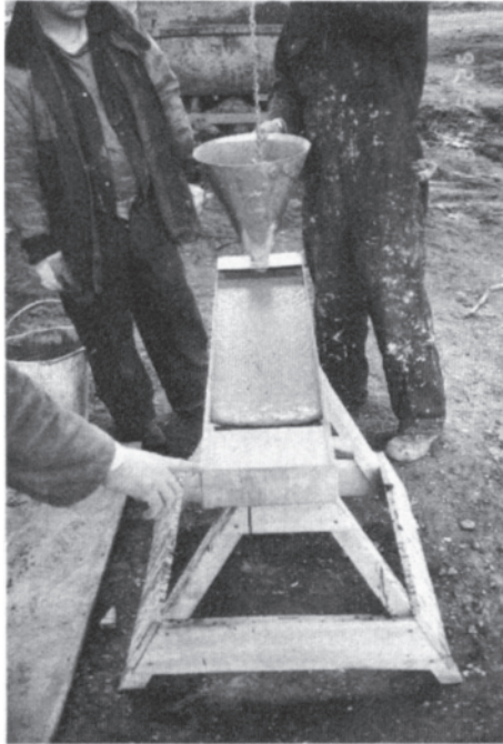
Figure 8.3 Assessment of flow characteristics with a flow test.
