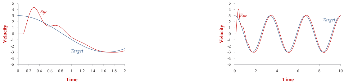
Figure 2.12: (Left) Smooth pursuit response with gain K = 10 . Response to steady state illustrating the transient response due to the oculomotor plant. (Right) Steady state response.
