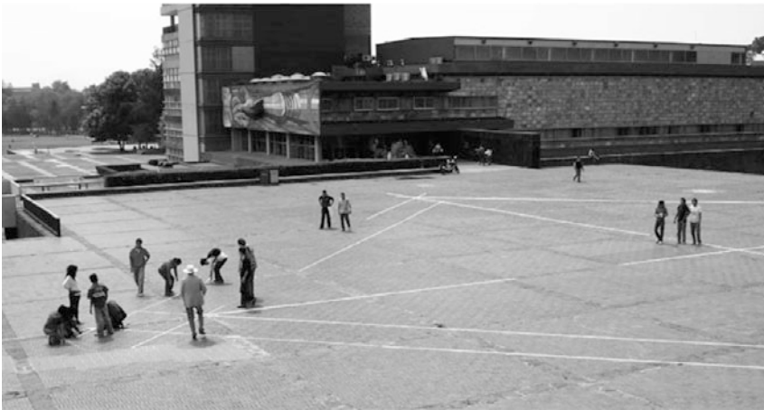
Fig. 14. Experiment to prove the feasibility of what I call the Mayan method for laying out a square. We laid out the base of the older pyramid, on campus, without using right angles.
