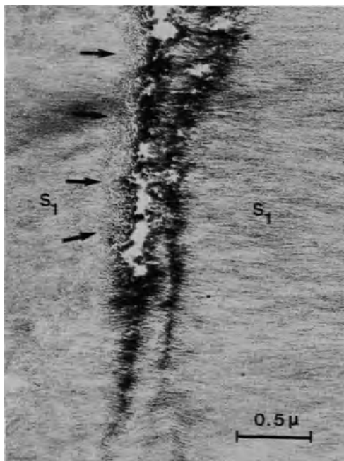
Figure 2. Lignin lamellae are changed in pattern from a layering in the wood to aggregates in the form of granula. The changes are seen to take place at a distance from the cell wall of the white-rot fungus Sporotrichum pulverulentum . From Ruel et al.(4).
