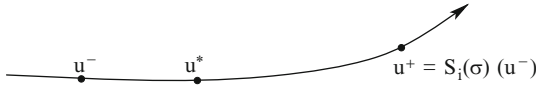
Fig. 16 The i -shock (u^-, u^+) satisfies the Liu admissibility conditions if its speed satisfies \lambda_i(u^-, u^+) \leq \lambda_i(u^-, u^*) for every intermediate state u^* along the i -shock curve through u^-
