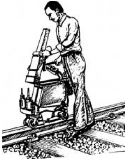
Fig. 6.8 Ultrasonic rail testing trolley
