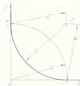
FIG. 12. An arc tangent at right-angle corner. The arc center must be equidistant from both lines.
