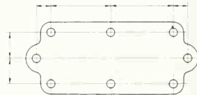
FIG. 79. Successive dimensioning. Tolerances accumulate.
