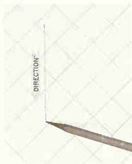
FIG. 69. Turning the paper to sketch an inclined line as a vertical line. This is often a great help because of the awkward position of the inclined line. An alternate turn is to the position of Fig. 71.
