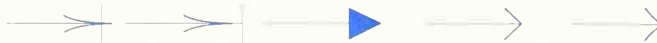
FIG. 5. Incorrect arrowheads. The first two examples show mistakes in placement. The last three illustrate shapes that are extremely poor.
