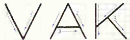
FIG. 9. The V-A-K group. The horizontal of A is one-third from the bottom; the second and third strokes of K are perpendicular to each other.
