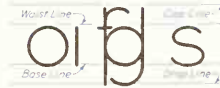
FIG. 18. Basic forms for lower-case letters. For standard letters, the waist-line height is two-thirds of capital height; capital line and drop line are therefore one-third above and one-third below the body of the letter.
