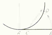
FIG. 58. To lay off, on an arc, a specified distance. See footnote 1 for accuracy.
