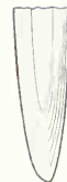
FIG. 51. Shape of worn pen nibs. This point needs sharpening to the shape of Fig. 48.
