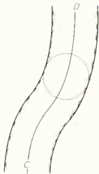
FIG. 93. Curved parallel lines. The curves are drawn tangent to circle arcs.
