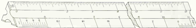
FIG. 8. An architect's (or mechanical engineer's) scale. Reduction in size is based on proportion of a foot.
