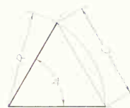
FIG. 31. Angle by chord. The proportion of C to R is obtained from a table of chords.
