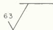
FIG. 96. Symbol. The roughness height rating is placed at the left of the long leg.
