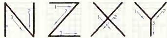
FIG. 8. The N-Z-X-Y group. Note that Z and X are smaller at the top than at the bottom, in accordance with the rule of stability.
