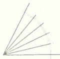
FIG. 35. To divide an angle into equal parts. Equal divisions (chords) are stepped off on an arc of the angle.
