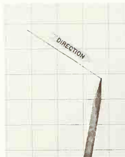
FIG. 70. Sketching an inclined line sloping downward from left to right. This is the most awkward position of any line. The paper should be turned as in Fig. 71 to aid in obtaining a smooth, accurate line.
