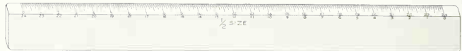
FIG. 6. A mechanical engineer's full- and half-size scale. Divisions are in inches to sixteenths of an inch. (The half-size scale is on the back of the full-size scale.)
