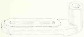
FIG. 83. Line-shading technique in pencil.
