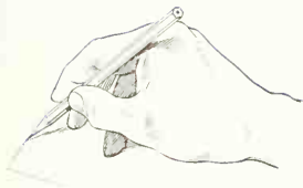
FIG. 64. Sketching a horizontal line. Draw from left to right with wrist pivot for short lines and forearm movement for long lines. Overlap strokes if necessary.
