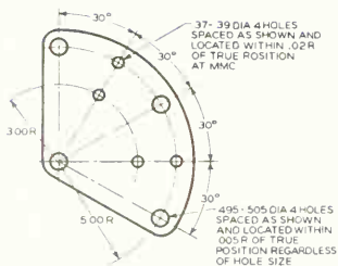
FIG. 89. True-position dimensioning (ANSI).
