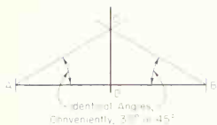
FIG. 22. To bisect a line (with T square and triangle). Equal angles locate one point on the perpendicular bisector.
