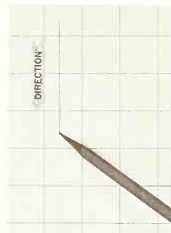
FIG. 67. Sketching a vertical line. Draw from top to bottom.
