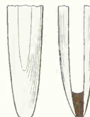
FIG. 50. Incorrect shape of pen nibs. This point is too flat. Ink will blob at the beginning and end of the line.
