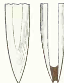
FIG. 49. Incorrect shape of pen nibs. This point is much too sharp. Ink will not flow well.
