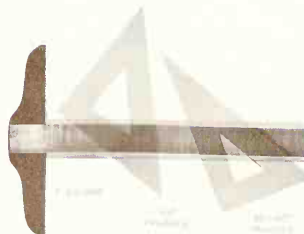
FIG. 5. T square and triangles. These are standard equipment for drawing straight lines.
