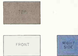
FIG. 1. Object faces parallel to the principal projection planes. Top, front, and side views are normal views, respectively, of top, front, and side of the object.
