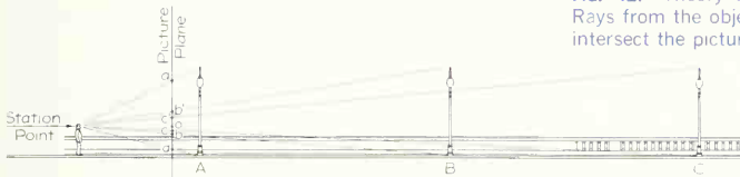
FIG. 43. The perspective drawing. This is the image formed on the picture plane of Fig. 42.
