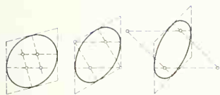
FIG. 36. Oblique circle construction. Note that the tangent points of arcs must be at the midpoints of the enclosing oblique square.
