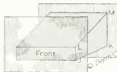
FIG. 21. Definition of depth. This is the difference from front to rear between two points.
