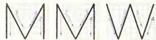
FIG. 10. The M-W group. M is one-twelfth wider than it is high; W is one-third wider than it is high.
