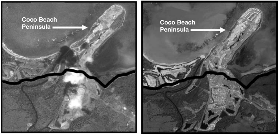
Figure 4.9 Comparison of the inland limits (black bold line) of a tsunami flood (maximum run up = 5.6 m) in the northern shore of the Municipality of Río Grande with built-up residential and commercial areas in 1999 (left) and 2010 (right).
