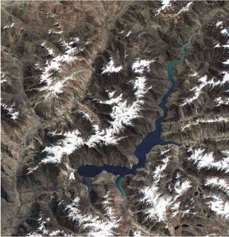
Fig. 1.3 Oblique photograph taken from International Space Station in September 2001 of Lake Sarez, Pamir Mountains, Tajikistan. Lake Sarez is a rockslide-dammed lake impounded by the 1911 Usoi rockslide (A) ([223]; Chap. 7 by Delaney and Evans, this volume). Lake Sarez has a length of ca. 60 km and a volume of ca. 17 \text{ Gm}^3 (NASA photograph ISS002-E-7524)
