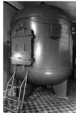
Fig. 25.1 Scheme of modeling equipment. 1 – Vacuum chamber (see on the right); 2 – Explosions simulators; 3 – Vacuum pump; 4 – Compressor; 5 – Vacuum-meter; 6 – Thermocouple vacuum-meter; 7 – Oil vacuum-meter; 8 – Differential valve; 9 – Mercury gage; 10 – Control and detonation device; 11 – Electromagnetic valve; 12 – High-speed camera
