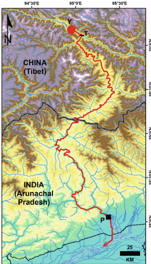
Fig. 22.1 Location of 2000 Yigong landslide dam (Y) and path of outburst flood (red line) resulting from the breach of the dam 62 days after emplacement. The flood followed the Yarlung Zangbo (Tibet) and Dihang (India) Rivers, and entered the main Brahmaputra below Pasighat (P) which is located 462 km downstream from the landslide dam. Tongmai Bridge (T) is a locality discussed in text
