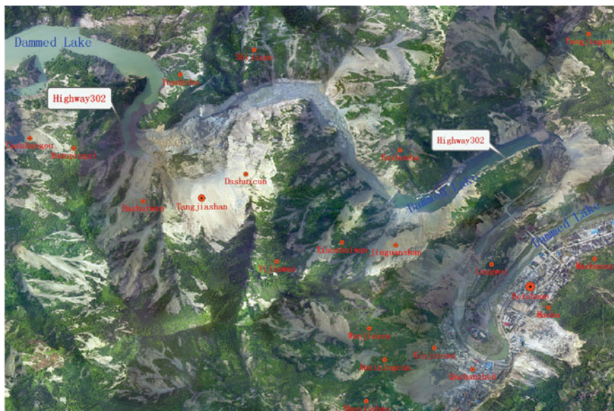
Fig. 10.6 The cluster of landslide dams along the major Tongkuo River Valley upstream from Beichuan County to the Tangjiashan rockslide dam. From left to right are the Tangjiashan dam, the Kuzhu landslide dam and the New – Street village landslide dam (Image from the Chinese Mapping Bureau)
