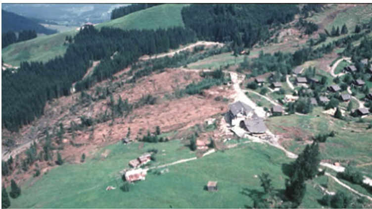
Fig. 3.10 Lower part of the Chlöwena landslide and the destroyed village of Falli Hölli. The lower part of the slide evolved in a mudslide to form a dam in the nearby river
