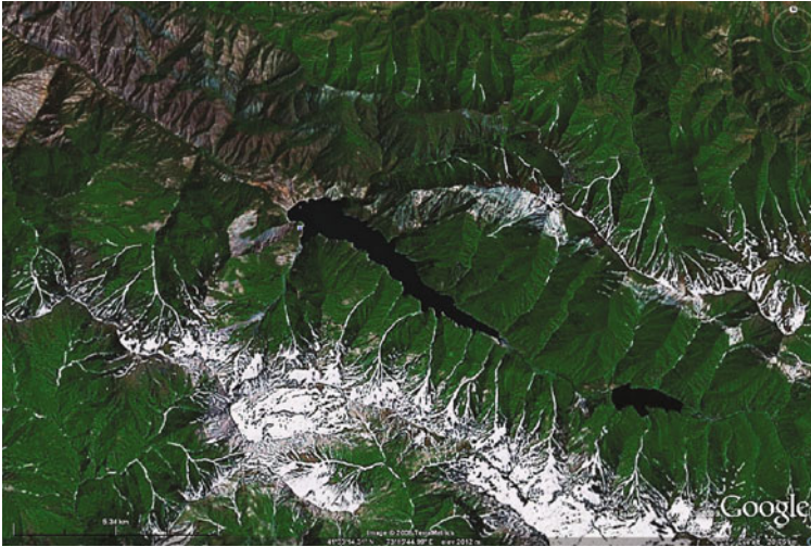
Fig. 1.4 Two rockslide-dammed lakes impounded by rockslides that have occurred along the linear trough marking the strike-slip Fergahna Fault, Kyrgyzstan (Google Earth image). The larger lake, Karasu Lake, is impounded by the Karasu rockslide (est. vol. 250 \text{ Mm}^3 ), the slide from the south side of the trough, as described by Strom [257, 258]
