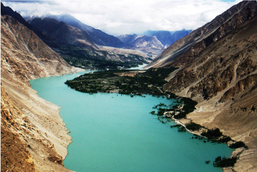
Fig. 7.12 Aerial view of 2010 Hunza rockslide-dammed lake in northern Pakistan. At the time of the photograph (May 13, 2010; Day 127 of impoundment) lake waters are still rising (pool el. 2,423 m a.s.l.), filling the Hunza Valley. View is upstream. Lake would rise another 12 m before overtopping on May 29, 2010 ( Pamir Times photograph)
