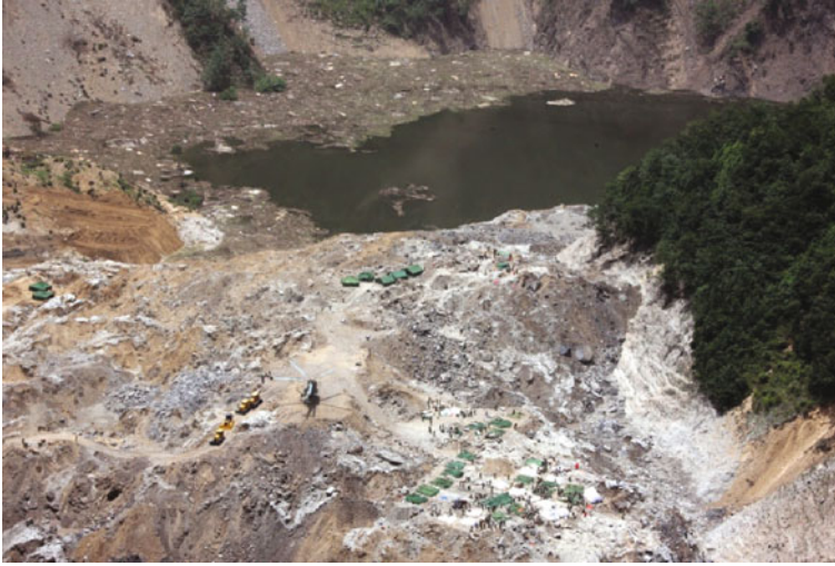
Fig. 1.20 Aerial view of Tangjiashan rockslide dam and lake forming upstream on May 28, 2010 (Day 16 of impoundment). Lake level was approximately 730 m a.s.l. and the lake volume was approaching 200 Mm 3 , approximately 81% of the maximum volume reached before controlled breaching on June 10, 2008 (photograph by Xinhua News Agency, China)
