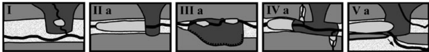
Fig. 24.1 Five main types (I–V) of plan view distribution of rockslide dams with letter representing sub-morphologies as described in the text and Figs. 24.2, 24.3, 24.4 and 24.5 (In this schematic figure as well as in the schematic Figs. 24.2, 24.3, 24.4, 24.5, 24.6 and 24.7 dark gray represents rockslide deposit, medium gray valley slopes, light gray lakes and dotted pattern the valley fill deposits)
