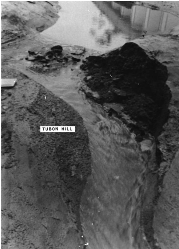
Fig. 14.9 Erosion in the physical scale model, view upstream, tested by EPN technical team [28]
