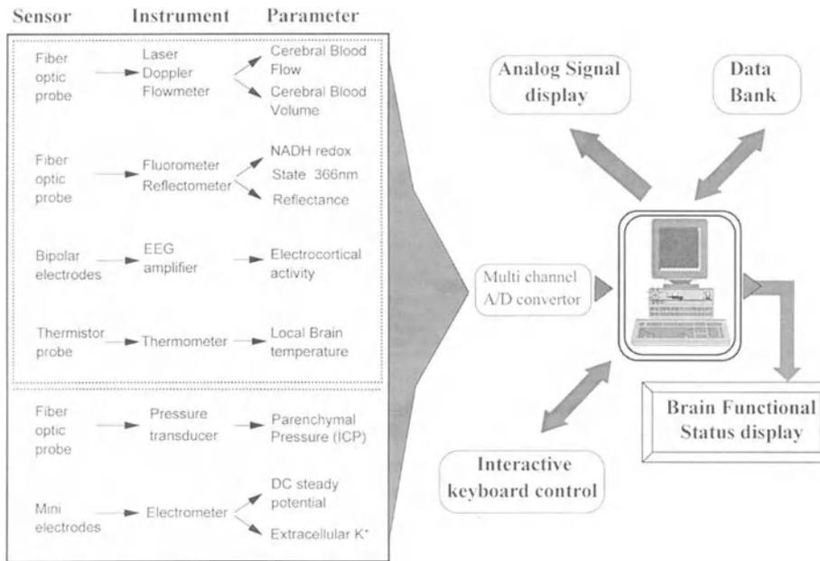
Fig. 1. Schematic presentation of the 2 multiparametric monitoring systems used in the operating room or in the Intensive Care Unit (ICU). The Brain Viability Analyzer (BVA) is based on the upper 4 sensors while by the addition of the other 3 (lower part) a total of 8 parameters were monitored
