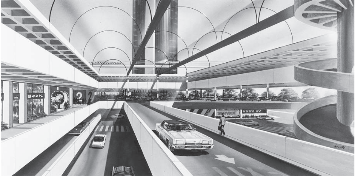
Concept drawing for parking substructure of Houston Center. An early publicity release stated that “Houston Center will recognize the relationship of the automobile to the Central Business District by providing adequate parking within the project area.” Four levels of parking were to be provided along the perimeter of the Phase One development. The master plan called for the eventual creation of 40,000–50,000 parking spaces. (Houston Center Vertical File, Courtesy HMRC, Houston Public Library.)
