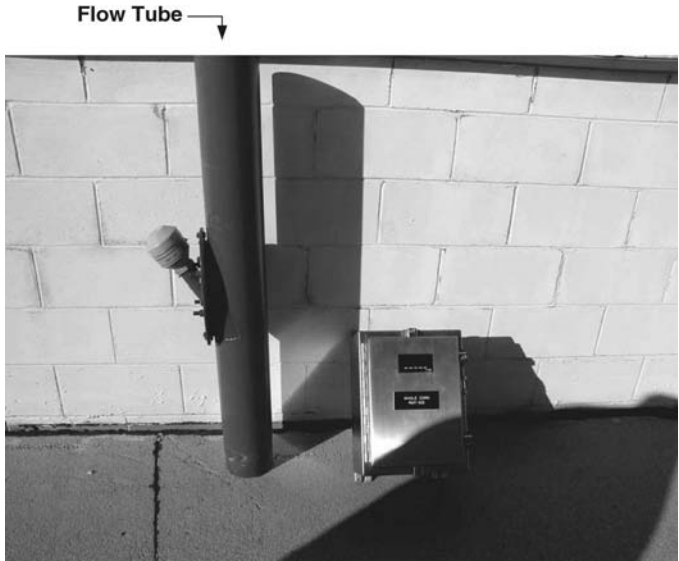
FIGURE 11.33 RayMas® Noncontact Solids Flow Meter, Gravity Flow Type; 6-inch Diameter Metering Whole Corn, Similar 8-inch Diameter Metering Ground Processed Corn.
