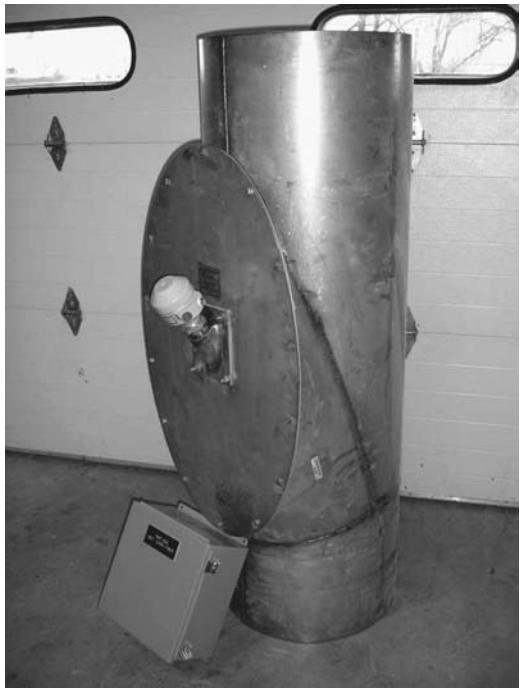
FIGURE 11.34 RayMas® Noncontact Solids Flow Meter, 20-inch Diameter, Gravity Flow Type, Product Material Metered—Wet Corn Material.
