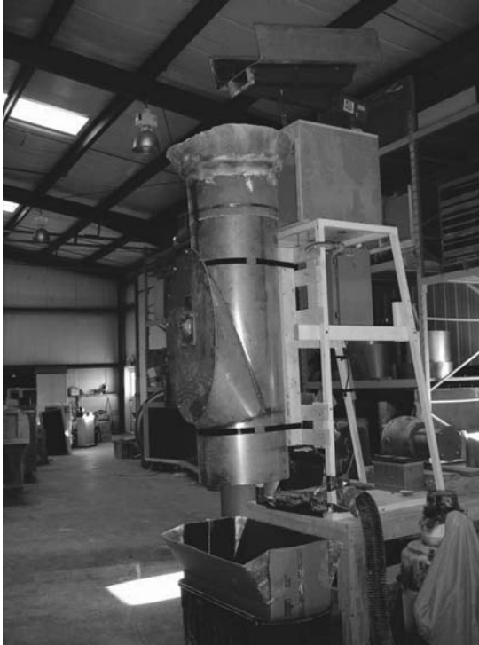
FIGURE 11.36 Calibration Equipment for a RayMas ® Solids Flow Meter, Gravity Flow Types.
