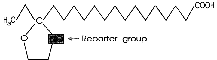
Fig. 1. Spin label 16-doxyl-stearic-acid with paramagnetic reporter group
