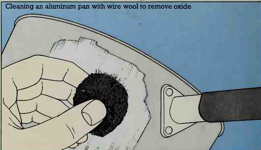
Cleaning an aluminum pan with wire wool to remove oxide
