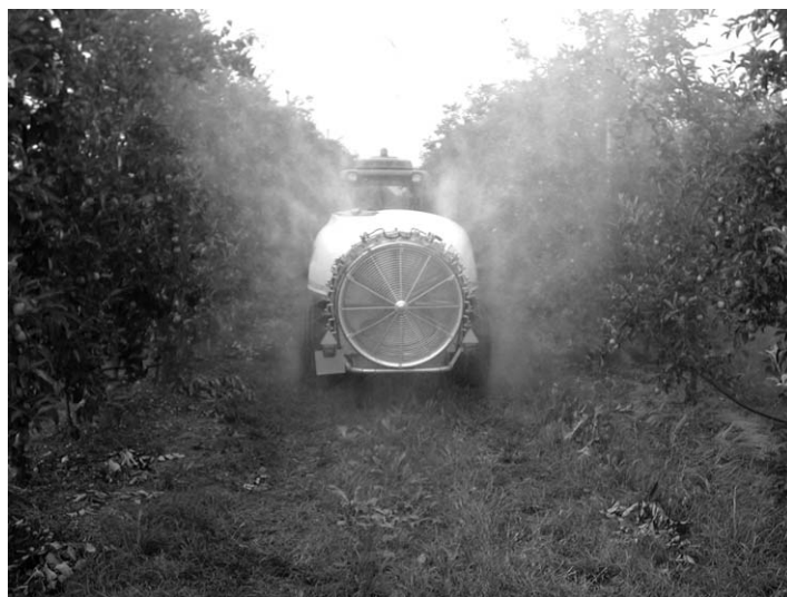
Figure 4 Axial-fan airblast sprayers are the most commonly used for foliar spray applications in apple orchards worldwide. This design is comparatively simple, low cost and flexible for use in a wide range of orchard structures but a large radial spray plume is generated which is prone to drift and losses to the soil.
